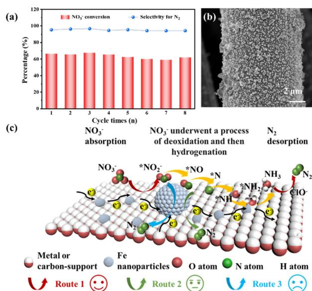
**Fig. 4** (a) Nitrate conversion and nitrogen selectivity of Fe/GF during 8 repeated electrolysis tests. (b) SEM images of Fe/GF after 8 cycles. (c) Reaction mechanism diagram of Fe/metal or carbon support in the bi-electrolyte (NaCl and  $\text{Na}_2\text{SO}_4$ ) system.
