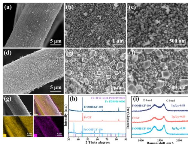
**Fig. 2** (a–c) SEM images of FeOOH/GF, (d–f) SEM images of Fe/GF, (g) EDX mapping image and the corresponding mapping scan images, (h) XRD patterns and (i) Raman spectra of Fe/GF with different calcination temperatures.
