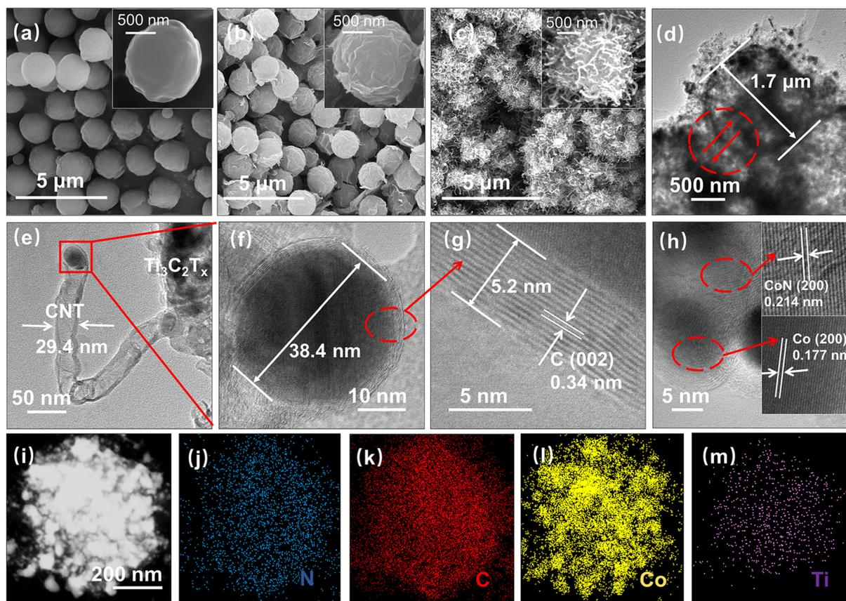
**Fig. 2** Scanning electron microscopy (SEM) images of PMMA (a),  $\text{Ti}_3\text{C}_2\text{T}_x/\text{PMMA}$  (b), and CoN-CNT@SMXene (c). (d and e) Transmission electron microscope (TEM) image of CoN-CNT@SMXene. (f–h) High-resolution TEM (HRTEM) images of CoN-CNT@SMXene. (i–m) Energy dispersive X-ray spectra (EDS) images of CoN-CNT@SMXene.
