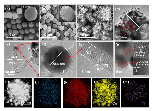
Fig. 2 Scanning electron microscopy (SEM) images of PMMA (a), Ti<sub>3</sub>C<sub>2</sub>T<sub>x</sub>/PMMA (b), and CoN-CNT@SMXene (c). (d and e) Transmission electron microscope (TEM) image of CoN-CNT@SMXene. (f-h) High-resolution TEM (HRTEM) images of CoN-CNT@SMXene. (i-m) Energy dispersive X-ray spectra (EDS) images of CoN-CNT@SMXene.
