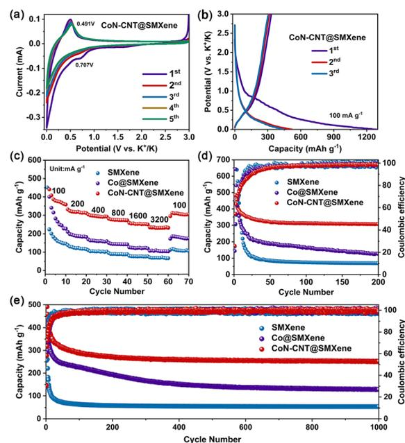
**Fig. 4** (a) CVs of CoN-CNT@SMXene at a scan rate of 0.1 mV s<sup>−1</sup>. (b) Discharge–charge profiles of CoN-CNT@SMXene at 0.1 A g<sup>−1</sup> at different cycles. (c) Rate capability of SMXene, Co@SMXene, and CoN-CNT@SMXene electrodes. Cycling performance of SMXene, Co@SMXene, and CoN-CNT@SMXene electrodes at (d) 0.1 A g<sup>−1</sup> for 200 cycles. (e) 0.4 A g<sup>−1</sup> for 1000 cycles.
