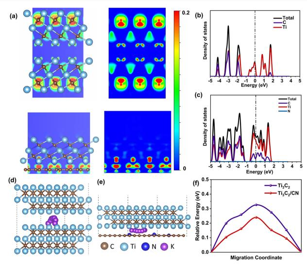
Fig. 6 (a) Charge density difference (CDD) of  $Ti_3C_2$  structure and the interfacial structure between  $Ti_3C_2$  and N-doped carbon. (b and c) Total and partial densities of states (DOSs) of  $Ti_3C_2$  and  $Ti_3C_2/CN$ . (d and e) The migration path of  $K^+$  in  $Ti_3C_2$  and  $Ti_3C_2/CN$ . (f)  $K^+$  migration coordinate of  $Ti_3C_2$  and  $Ti_3C_2/CN$ .
