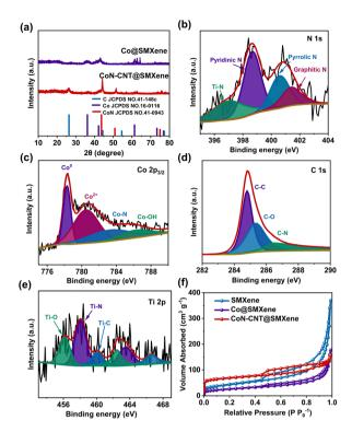
Fig. 3 (a) XRD patterns of Co@SMXene and CoN-CNT@SMXene. (b-e) High-resolution N 1s (b), Co 2p (c), C 1s (d) and Ti 2p (e) XPS spectra of CoN-CNT@SMXene. (f) N<sub>2</sub> adsorption/desorption isotherms.
