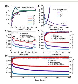
Fig. 4 (a) CVs of CoN-CNT@SMXene at a scan rate of 0.1 mV  $s^{-1}$ . (b) Discharge-charge profiles of CoN-CNT@SMXene at 0.1 A  $\rm g^{-1}$  at different cycles. (c) Rate capability of SMXene, Co@SMXene, and CoN-CNT@SMXene electrodes. Cycling performance of SMXene, Co@SMXene, and CoN-CNT@SMXene electrodes at (d)  $0.1 \text{ A g}^{-1}$  for 200 cycles. (e)  $0.4 \text{ A g}^{-1}$  for 1000 cycles.
