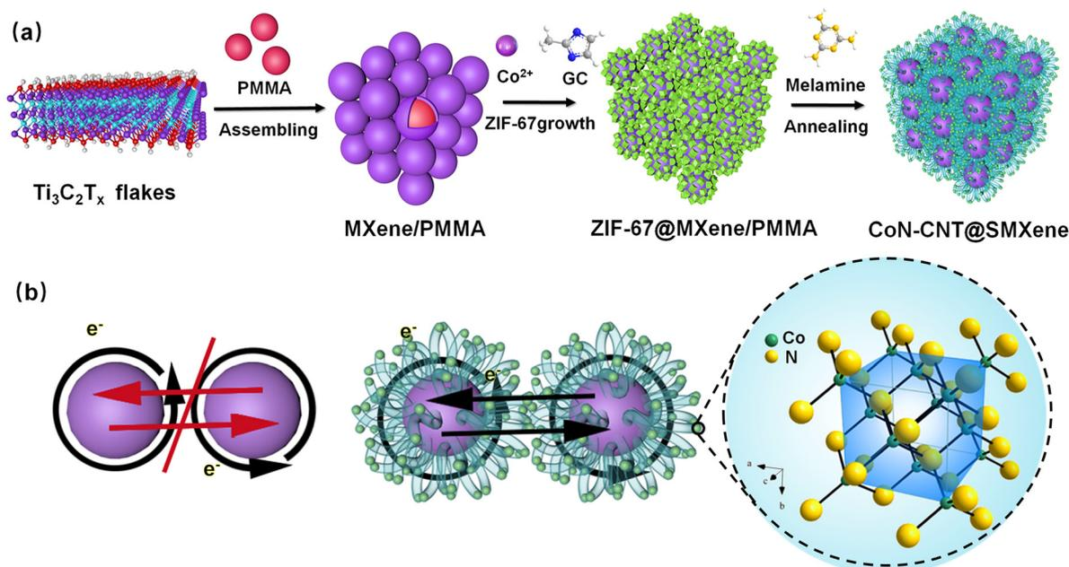
Fig. 1 (a) Schematic illustration of the synthesis process of CoN-CNT@SMXene. (b) Schematic illustrating electron transfer in CoN-CNT@SMXene.
