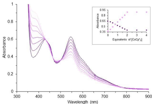
**Fig. 3** Reduction of 0.1 mM **1** in THF by addition of  $\text{CoCp}^*_2$  in increments of 0.25 equiv. as monitored by UV-vis spectroscopy (path length, 1.0 cm). Inset: corresponding changes of the absorbance at 389 (◆) and 545 (●) nm.
