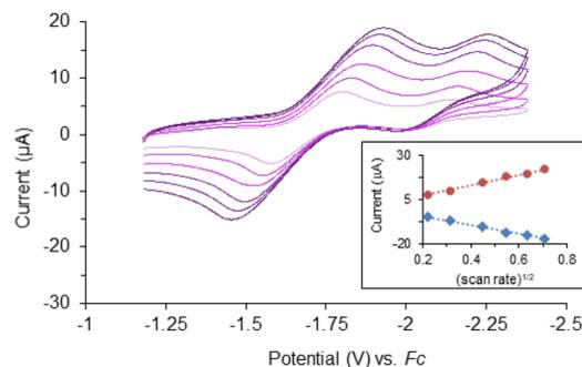
**Fig. 2** Overlaid cyclic voltammograms of **1** (1 mM) in THF with 0.1 M N(Bu)<sub>4</sub>PF<sub>6</sub>. Scan rates = 50, 100, 200, 300, 400, 500 mV s<sup>-1</sup> referenced to a ferrocene/ferrocenium redox couple (Fc). Inset: plot of cathodic peak current (●, R<sup>2</sup> = 0.9953) and anodic peak current (◆, R<sup>2</sup> = 0.9962) versus square root of scan rate.
