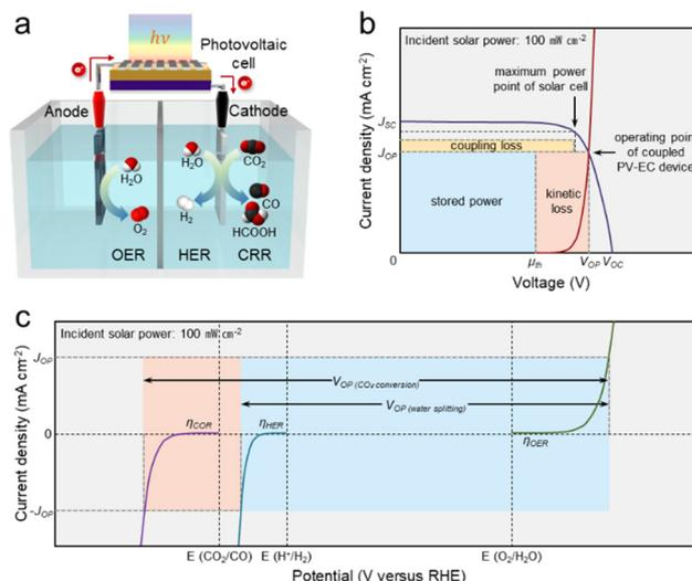
**Fig. 1** The principles of photovoltaic-electrochemical (PV-EC) device. (a) Schematic of PV-EC cell. (b) The generalized current density-voltage ( $J$ - $V$ ) diagram (2-electrode measurement) of a directly coupled PV-EC device. Reproduced from ref. 13. Copyright 2013 PNAS. (c) The generalized  $J$ - $V$  diagrams (3-electrode measurement) of anode and cathode for electrochemical reactions (water splitting and CO<sub>2</sub> conversion).
