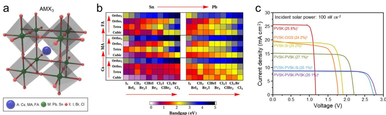
**Fig. 3** Halide perovskite-based solar cells. (a) General crystal structure (AMX<sub>3</sub>) of the halide perovskite. (b) Calculated band gaps of halide perovskites with different composition and phase. Reproduced from ref. 43. Copyright 2014 AIP Publishing. (c) J–V curves of various halide perovskite tandem solar cells with benchmarked power conversion efficiencies (PCE). Benchmark list: (1) ref. 55, (2) ref. 46, (3) ref. 54, (4) ref. 53, (5) ref. 52, (6) ref. 56
