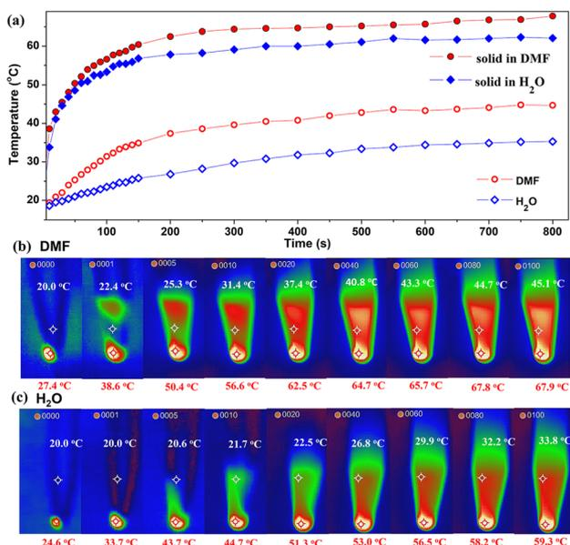
**Fig. 8** Photothermal experiment in solvent for Cu<sub>12</sub> (a) time-temperature curves; photothermal images in DMF (b) and H<sub>2</sub>O (c). Red and white labels represent sample and solvent temperatures.
