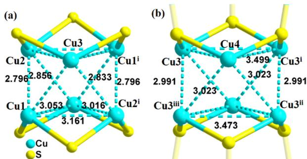
Fig. 2 (a)  $\text{Cu}\cdots\text{Cu}$  distance (Å) in  $\text{Cu}_6$  and (b)  $\text{Cu}\cdots\text{Cu}$  distance (Å) in the “ $\text{Cu}_6(2\text{-PyS})_6$ ” core of  $\text{Cu}_{12}$ . Symmetry codes:  $\text{Cu}_6$  (i)  $-x + 1, -y + 1, -z + 1$ ;  $\text{Cu}_{12}$  (i)  $x, y, -z + 1$ ; (ii)  $-x + 1, -y + 1, -z + 1$ ; (iii)  $-x + 1, -y + 1, z$ .
