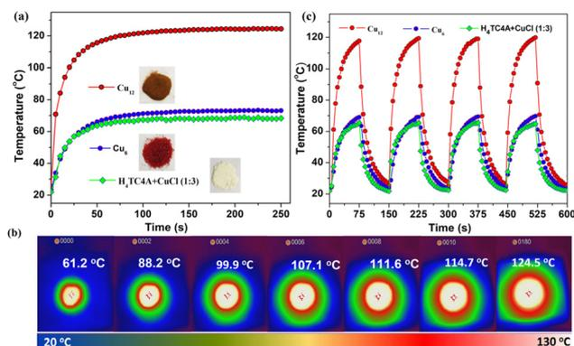
Fig. 7 Photothermal experiment in the solid state: (a) time–temperature curves for  $\text{Cu}_{12}$ ,  $\text{Cu}_6$ , and the mixture; (b) photothermal images for  $\text{Cu}_{12}$  (interval, 5 s); (c) light on–off cycles.
