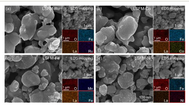
Fig. 2 Scanning electron microscopy (SEM) images and EDS mapping results taken for (a) LSFM-Ru, (b) LSFM-Co, (c) LSFM-Fe, and (d) LSFM-Ni electrodes after sintering at 1073 K.
