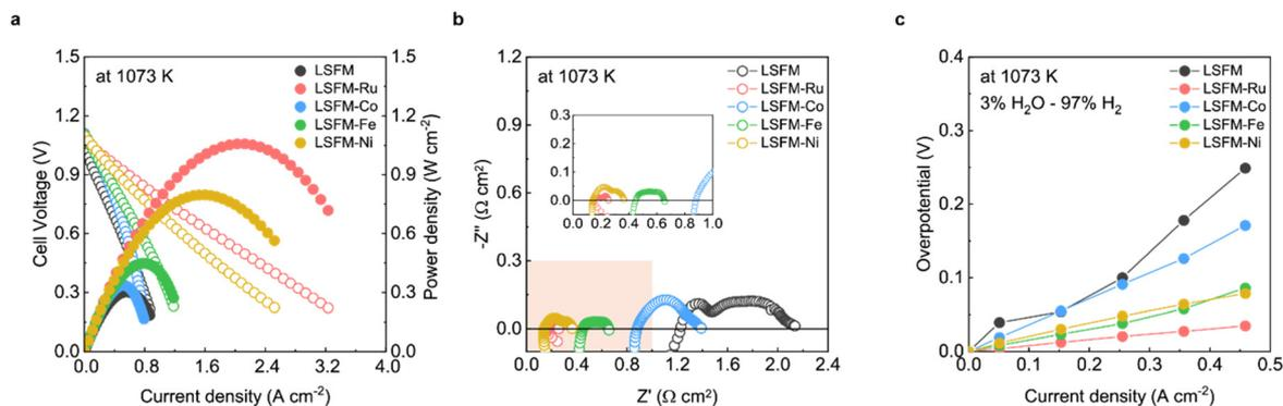
**Fig. 3** (a) The I-V curves and (b) the impedance data of single cells of LSFM and infiltrated LSFM electrodes (Co, Fe, Ni, and Ru) at 1073 K under H<sub>2</sub>O : H<sub>2</sub> (3%:97%). (c) The polarization overpotential is calculated from the impedance data.
