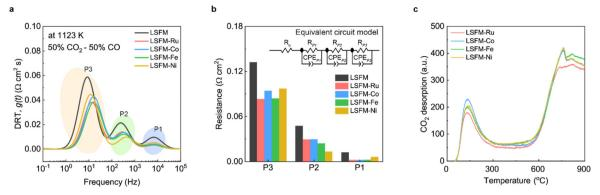
Fig. 6 (a) Comparison of plots of the distribution of relaxation times (DRT) for LSFM and the infiltrated LSFM electrodes at 1123 K. (b) Polarization resistance of each cell calculated from the circuit model fitting results, and (c) the CO2-TPD profiles of the metal infiltrated LSFM.
