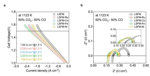
Fig. 4 (a) The  $CO_2$  electrolysis performance with the infiltrated LSFM electrode feeding  $CO_2$ : CO (50:50) at 1123 K. (b) Total impedance spectra of the cell with the infiltrated LSFM electrode at 1123 K.
