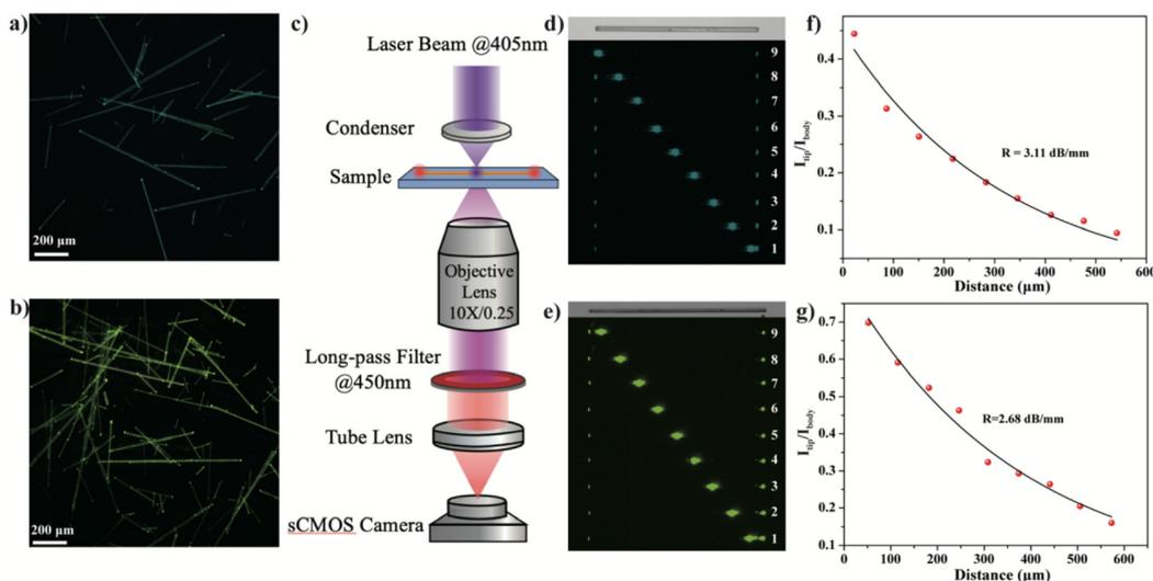
**Fig. 5** PL microscope images of (a) 1-C5 and (b) 1-C7 under unfocused UV light (365 nm). (c) Schematic illustration of the optical waveguide test. PL microscope images of (d) 1-C5 and (e) 1-C7 for the optical waveguide test under the excitation of 405 nm continuous laser at different positions. The correlation of the  $I_{\text{tip}}/I_{\text{body}}$  with the photon propagation distance for (f) 1-C5 and (g) 1-C7.
