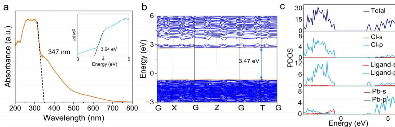
Fig. 2 (a) UV-vis diffuse reflectance spectroscopy of TJU-19. The inset shows the estimated band gap according to the Tauc plot. (b) The calculated band structure of TJU-19. (c) pDOS of TJU-19.
