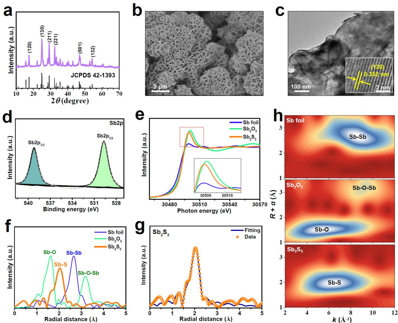
**Fig. 1** Characterization of  $\text{Sb}_2\text{S}_3$ : (a) XRD pattern, (b) SEM image, (c) TEM image and HRTEM image (inset), (d) XPS  $\text{Sb}2p$  spectrum, (e) Sb K-edge XANES spectra, (f) EXAFS spectra and (h) WT profiles of  $\text{Sb}_2\text{S}_3$  and reference samples. (g) EXAFS fitting curve of  $\text{Sb}_2\text{S}_3$ .
