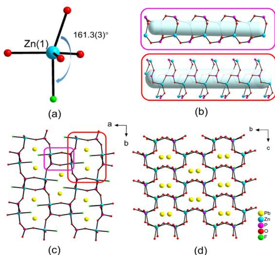
**Fig. 1** The ZnO<sub>4</sub>F triangular bipyramid (a), the 1D four-MPR channel (purple rectangle) and the eight-MPR channel (red rectangle) (b), the 3D structure of PbZn(PO<sub>4</sub>)F along the *c*-axis (c) and the *a*-axis (d) (the Pb–O and Pb–F bonds have been neglected for clarity).
