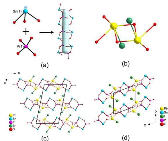
**Fig. 2** The SnO<sub>3</sub> group, PO<sub>4</sub> group and [Sn(PO<sub>4</sub>)<sub>2</sub>]<sup>4–</sup> chain (a), Pb<sub>2</sub>O<sub>6</sub>X<sub>2</sub> dimer (b), the framework of PbSn(PO<sub>4</sub>)Br (c) and PbSn(PO<sub>4</sub>)I (d).
