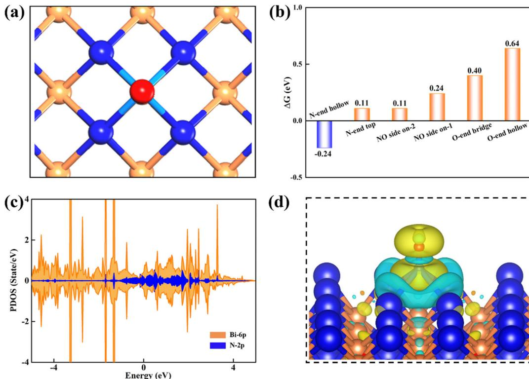
**Fig. 2** (a) The optimized configuration, (b) the adsorption free energies ( $\Delta G$ ) for NO adsorption on the  $\beta$ -PdBi<sub>2</sub> monolayer in various possible adsorption patterns, (c) the projected density of states (PDOS) and (d) the charge difference density of the  $\beta$ -PdBi<sub>2</sub> monolayer with an isovalue of  $0.003 \text{ e} \text{ \AA}^{-3}$  (before and after NO adsorption). Cyan and yellow bubbles represent positive and negative charges, respectively.
