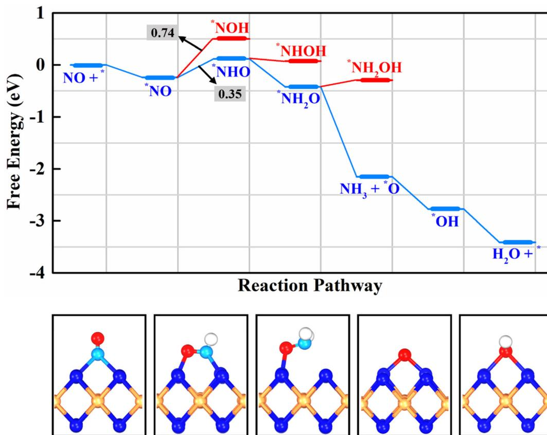
Fig. 4 The energetically most favorable free energy profile for the electroreduction of NO molecules to  $\text{NH}_3$  product on the  $\beta\text{-PdBi}_2$  monolayer and the involved reaction intermediates. The blue, orange, red, light blue, and white spheres represent the Bi, Pd, O, N, and H atoms, respectively.
