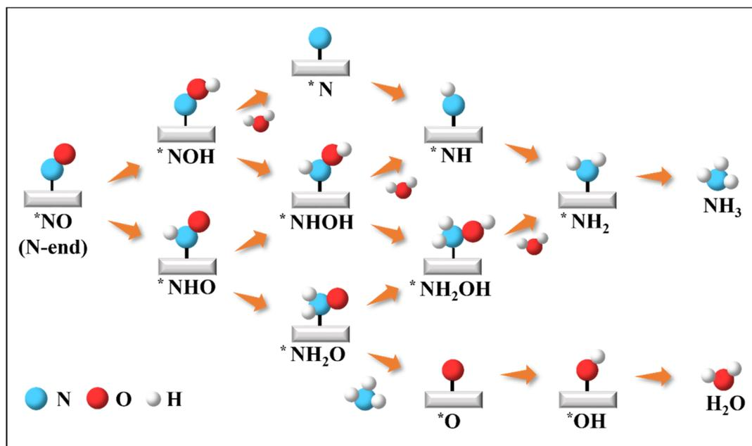
Fig. 3 Schematic depiction of all possible pathways for electrocatalytic NORR to NH<sub>3</sub> along the N-end pathway on the  $\beta$ -PdBi<sub>2</sub> monolayer.
