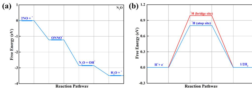
Fig. 5 (a) The energetically most favorable free energy profile for the electroreduction of 2NO molecules to the  $\text{N}_2\text{O}$  product on the  $\beta\text{-PdBi}_2$  monolayer and (b) the calculated Gibbs free profile of HER on the  $\beta\text{-PdBi}_2$  monolayer.
