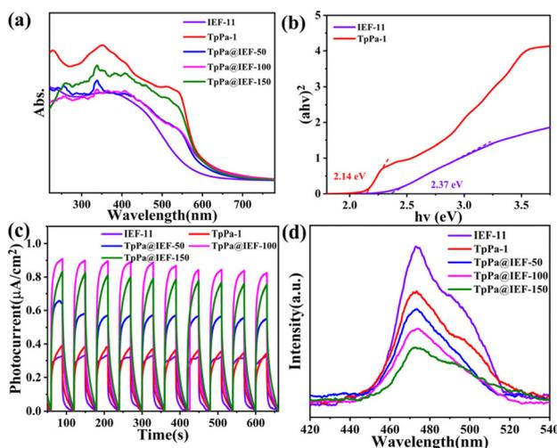
**Fig. 4** (a) UV-vis absorption spectra of **IEF-11**, **TpPa-1** and **TpPa@IEF-X**; (b) band gaps of **IEF-11** and **TpPa-1**; (c) transient photocurrent response graphs of **TpPa-1**, **IEF-11** and **TpPa@IEF-X**; and (d) photoluminescence spectra of **TpPa-1** and **TpPa@IEF-X**.
