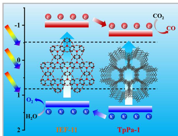
Fig. 6 The mechanism of  $\text{CO}_2$  photoreduction by **TpPa@IEF-X**.
