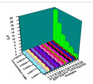
Fig. 6 3D Stern-Volmer plot for the detection of Hg<sup>2+</sup>.
