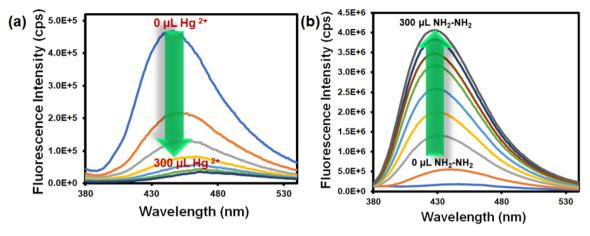
Fig. 2 Change in the fluorescence emission intensity of the probe Hf-UiO-66-NHCSNHCH<sub>3</sub> after the incremental addition of 300 µL aqueous 10 mM Hg<sup>2+</sup> (a) and NH<sub>2</sub>-NH<sub>2</sub> (b) solution.
