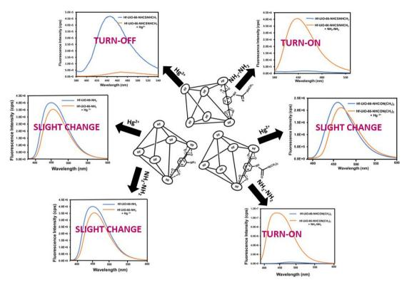
Fig. 9 Schematic representation of the change in the fluorescence emission intensity of Hf-UiO-66-NHCSNHCH<sub>3</sub>, Hf-UiO-66-NH<sub>2</sub>, and Hf-UiO-66-NHCON(CH<sub>3</sub>)<sub>2</sub> before and after the addition of Hg<sup>2+</sup> and NH<sub>2</sub>-NH<sub>2</sub>.
