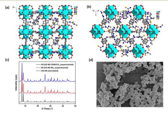
Fig. 1 (a) and (b) Simulated structure of Hf-UiO-66-NHCSNHCH<sub>3</sub> with Hf atoms shown as cyan polyhedra. (c) Comparative PXRD pattern of Hf-UiO-66-NHCSNHCH<sub>3</sub> with Hf-UiO-66-NHCSNHCH<sub>3</sub> and UiO-66 MOF (simulated), (d) FE-SEM image of Hf-UiO-66-NHCSNHCH<sub>3</sub>.
