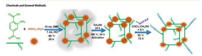
Scheme 1 Detailed stepwise synthesis of Hf-UiO-66-NHCSNHCH<sub>3</sub>.
