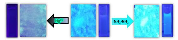
Fig. 8 Naked eye detection of  $Hg^{2+}$  and  $NH_2-NH_2$  by MOF-coated cotton composite under a fluorescence lamp.
