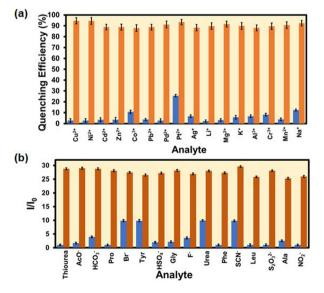
Fig. 5 The comparative selectivity bar plot (with standard deviations) of probe Hf-UiO-66-NHCSNHCH<sub>3</sub> toward Hg<sup>2+</sup> (a) and NH<sub>2</sub>-NH<sub>2</sub> (b) in the presence of their respective congeners. The brown bars represent the quenching efficiency toward Hg2+ and fold increment in the case of  $NH_2-NH_2$  and the blue bars belong to the competitive analytes.
