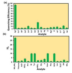
Fig. 4 Comparative selectivity bar plots of the probe Hf-UiO-66-NHCSNHCH<sub>3</sub> toward Hg<sup>2+</sup> (a) and NH<sub>2</sub>-NH<sub>2</sub> (b) with their respective are congeners (plots shown with standard deviations 3 measurements)
