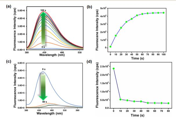
Fig. 3 Time-dependent fluorescence emission intensity of probe Hf-UiO-66-NHCSNHCH<sub>3</sub> after the addition of 300 µL 10 mM aqueous solution of  $NH_2-NH_2$  (a) and  $Hg^{2+}$  (c). Fluorescence intensity versus time plot for  $NH_2-NH_2$  (b) and  $Hg^{2+}$  (d).
