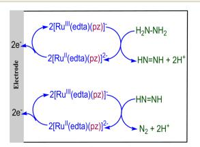
Electrochemical oxidation of N<sub>2</sub>H<sub>4</sub> to N<sub>2</sub> catalyzed by [Ru<sup>III</sup>(edta) Fig. 4 (pz)]-.
