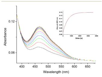
Fig. 3 Spectral changes that occurred for the reaction of [Ru<sup>III</sup>(edta) (pz)] with hydrazine (N2H4).
