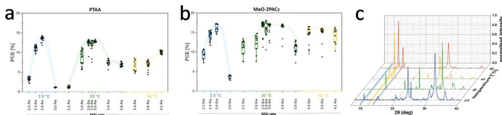
**Fig. 7** Box plot of power conversion efficiency extracted from  $J-V$  scans (reverse and forward) measured under simulated AM 1.5G illumination for solar cells prepared at different substrate temperatures and MAI rates on (a) PTAA and (b) MeO-2PACz. (c) Normalized XRD patterns of co-evaporated films on PTAA deposited with different substrate temperatures. Reproduced with permission.<sup>101</sup> Copyright 2020, American Chemical Society.
