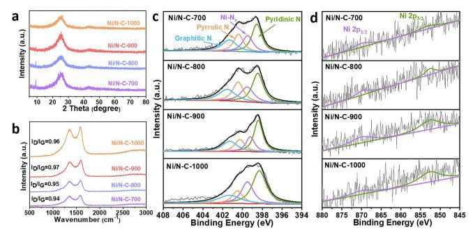
Fig. 2 (a) XRD patterns and (b) Raman spectra of various Ni/N-C catalysts. High-resolution XPS spectra of (c) N 1s and (d) Ni 2p in Ni/N-C-700, 800, 900 and 1000.
