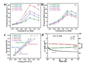
Fig. 4 (a) CO and (b) H<sub>2</sub> production rates of Ni/N-C catalysts at different applied potentials. (c) Tafel plots based on  $j_{CO}$  of the Ni/N-C catalysts in CO<sub>2</sub>-saturated 0.1 M KHCO<sub>3</sub> solution. (d) Long-term stability test of Ni/N-C-900 at -0.8 V vs. RHE for 10 h.
