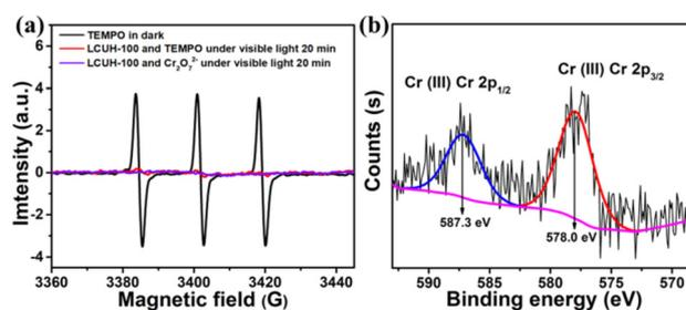
Fig. 7 (a) EPR signal of TEMPO in the dark, and TEMPO and  $Cr_2O_7^{2-}$  radicals under visible light in aqueous dispersion of **LCUH-100** for 20 min; (b) XPS spectra of the recovered **LCUH-100** after the Cr(VI) reduction experiment.
