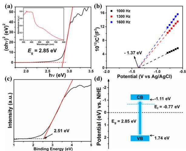
**Fig. 4** (a) UV-vis spectra of LCUH-100 and plot of  $(ah\nu)^2$  versus photon energy ( $h\nu$ ) of LCUH-100. Typical Mott-Schottky plots (b) and XPS VB spectra (c) of LCUH-100. (d) Band structure diagram of LCUH-100.
