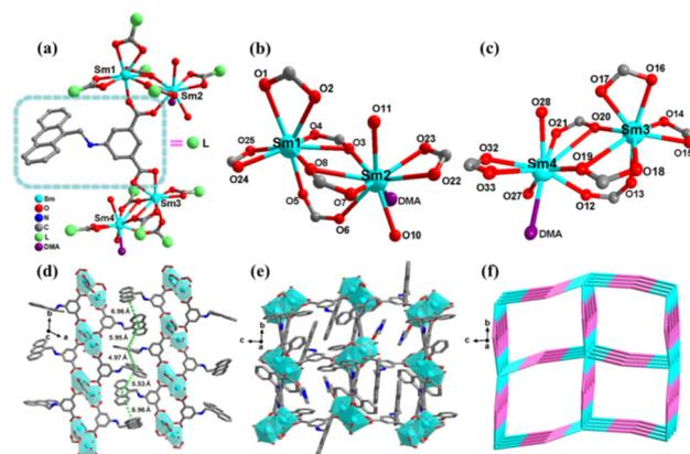
**Fig. 1** (a) Simplified coordination environments of **LCUH-100** (green spheres represent H<sub>2</sub>AAPA). Coordination structures of binuclear [Sm<sub>2</sub>(COO)<sub>6</sub>]<sup>a</sup> (b) and binuclear [Sm<sub>2</sub>(COO)<sub>6</sub>]<sup>b</sup> (c). (d) Lamellar structure of the 2D framework viewed from the c axis. (e) Reticular structure viewed from the a axis in **LCUH-100**. (f) Simplified topology structure of **LCUH-100**.
