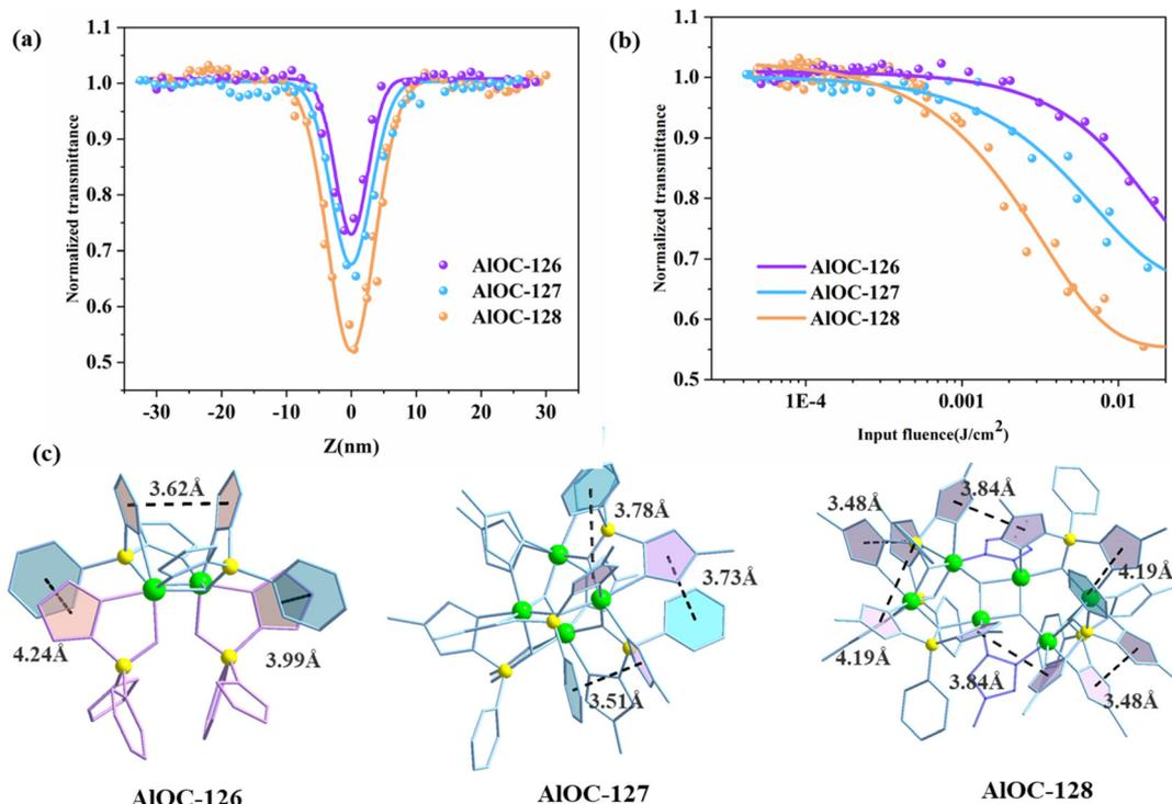
**Fig. 6** (a) OA Z-scan curves and (b) OL curves of the samples at picosecond laser excitation (input energy: 4  $\mu\text{J}$ ). The linear transmittance of the samples was adjusted to be 65%. Colored scattered balls indicate experimental data with the solid line representing the curve of best fit. (c)  $\pi\cdots\pi$  interactions between adjacent L in **AIOC-126**, **AIOC-127**, and **AIOC-128**. Color code: Al, green; B, yellow.
