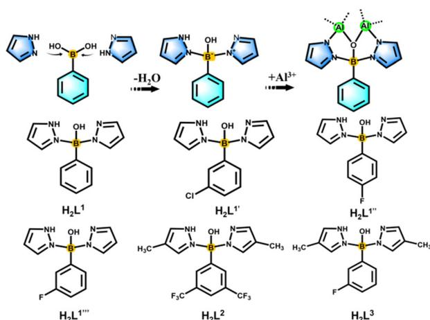
**Scheme 1** Reaction herein involving both *in situ* generated covalent bond and coordinate bond with  $Al^{3+}$ . Although these ligands cannot be isolated, we have listed them in detail in order to give a clearer picture of the ligands on each compound and the universality of the *in situ* reaction.
