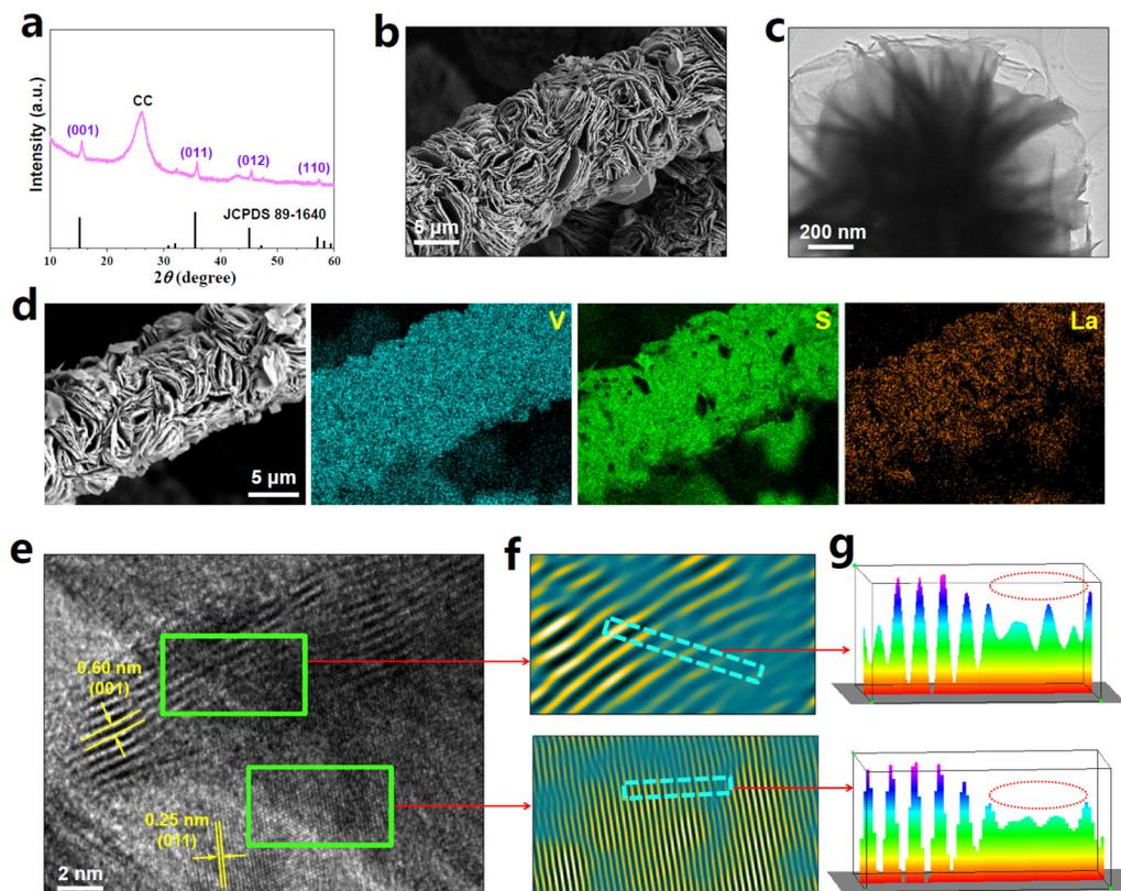
**Fig. 1** (a) XRD pattern of La- $\text{VS}_{2-x}$  on CC. (b) SEM image of La- $\text{VS}_{2-x}$  on CC. (c) TEM image of La- $\text{VS}_{2-x}$ . (d) Elemental mapping images of La- $\text{VS}_{2-x}$  on CC. (e) HRTEM image of La- $\text{VS}_{2-x}$  and (f) the corresponding IFFT pattern and (g) lattice line scanning analyses.
