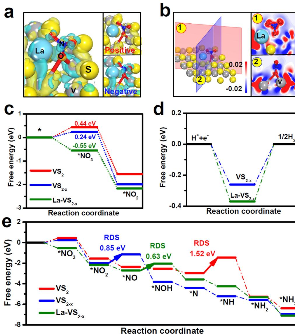
Fig. 4 (a) Differential charge density maps of  $\text{NO}_3^-$  adsorption on  $\text{La-VS}_{2-x}$  (yellow: accumulation, cyan: depletion) and (b) the corresponding electron location function maps (red: accumulation, blue: depletion). (c and d) Binding free energies of (c)  $\text{NO}_3^-$  and (d) H on different catalysts. (e) Gibbs free energy diagrams of the  $\text{NO}_3\text{RR}$  pathway of  $\text{VS}_2$ ,  $\text{VS}_{2-x}$  and  $\text{La-VS}_{2-x}$ , respectively.
