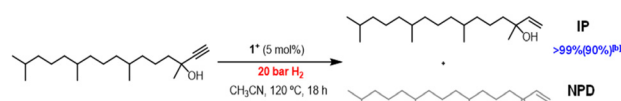
Fig. 6 Semihydrogenation of DIP. Reaction conditions: 0.1 mmol alkyne, 5 mol% catalyst, 20 bar H 2 , 120 °C, CH 3 CN (2 mL), 18 h. Conversions and yields determined by GC analysis using n -hexadecane as an internal standard.
