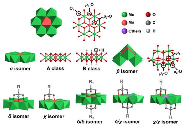
**Fig. 1** Structures and isomeric species of Anderson-type POMs, and isomeric species after modification with triol ligands. Color code:  $\{MoO_6\}$ , green octahedron;  $\{MnO_6\}$ , red octahedron;  $\{XO_6\}$ , violet octahedron ( $X =$  others). Hydrogen atoms in organic ligands have been omitted for clarity.
