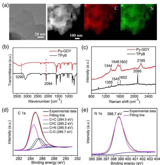
**Fig. 2** (a) TEM and EDS mapping images of **Py-GDY**. (b) FTIR spectra of **Py-GDY** and **TPyB**. (c) Raman spectra of **Py-GDY** and **TPyB**. (d) C 1s XPS spectrum, and (e) N 1s XPS spectrum of **Py-GDY**.
