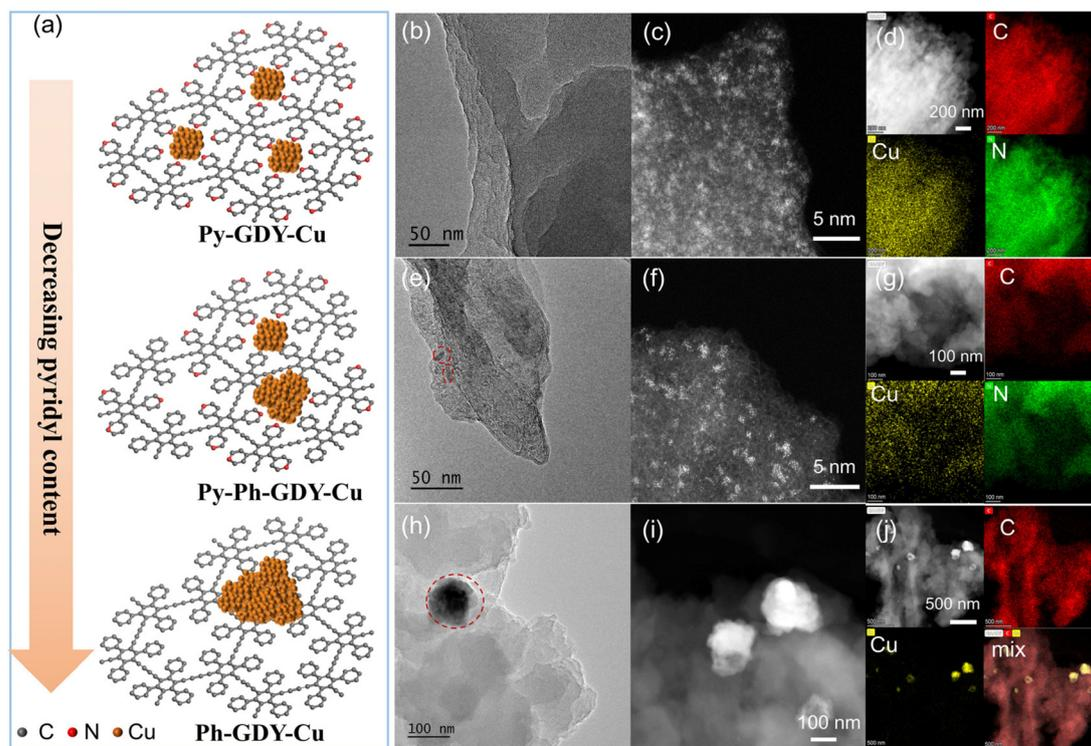
**Fig. 3** (a) Schematic illustration of **Py-GDY-Cu**, **Py-Ph-GDY-Cu**, and **Ph-GDY-Cu**. (b) TEM image, (c) aberration-corrected HAADF-STEM image, and (d) EDS mapping images of **Py-GDY-Cu**. (e) TEM image, (f) aberration-corrected HAADF-STEM image, and (g) EDS mapping images of **Py-Ph-GDY-Cu**. (h) TEM image, (i) HAADF-STEM image, and (j) EDS mapping images of **Ph-GDY-Cu**.
