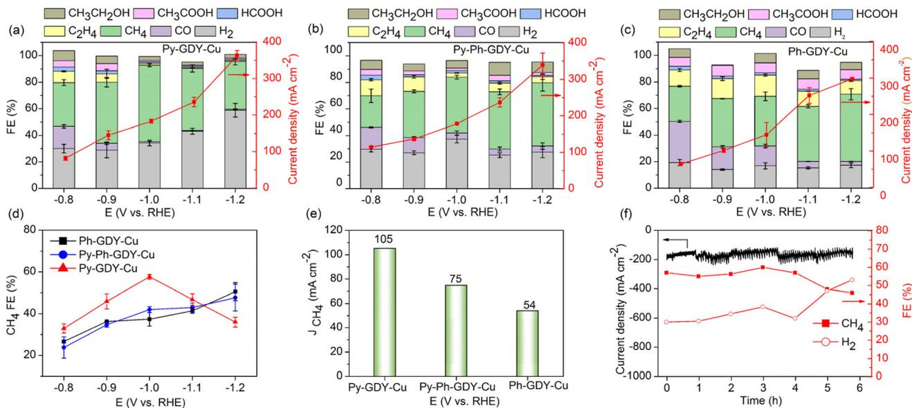
**Fig. 5**  $\text{CO}_2$  electroreduction performances of (a) **Py-GDY-Cu**, (b) **Py-Ph-GDY-Cu**, (c) **Ph-GDY-Cu** in 1.0 M KOH. (d) FE of  $\text{CH}_4$  at  $-0.8$  V to  $-1.2$  V vs. RHE. (e) Partial current density of  $\text{CH}_4$  at  $-1.0$  V vs. RHE. (f) Stability test of **Py-GDY-Cu** and the FE of  $\text{CH}_4$ ,  $\text{H}_2$  measured every 1 h at  $-1.0$  V vs. RHE.
