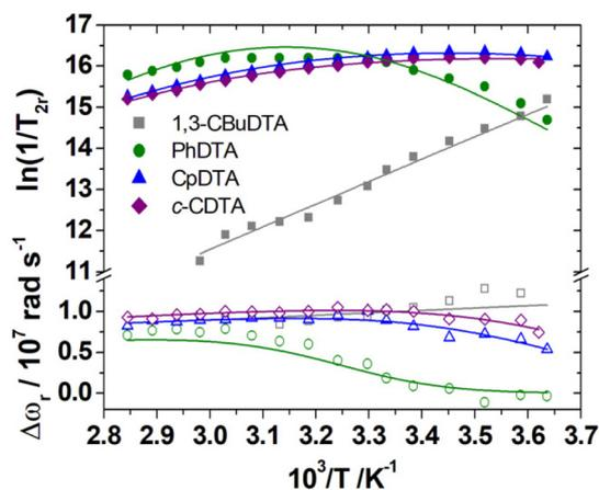
Fig. 7 Reduced  $^{17}\text{O}$  NMR transverse relaxation rates ( $1/T_{2r}$ , filled symbols) and chemical shifts ( $\Delta\omega_r$ , open symbols) measured for  $[\text{Fe}(c\text{-CDTA})]^-$  (3.2 mM, pH 5.9),  $[\text{Fe}(\text{CpDTA})]^-$  (5.9 mM, pH 6.1),  $[\text{Fe}(\text{PhDTA})]^-$  (4.9 mM, pH 7.2) and  $[\text{Fe}(\text{CBuDTA})]^-$  (3.9 mM, pH = 5.5) at 11.75 T. The solid lines represent the fits of the data, as described in the text.
