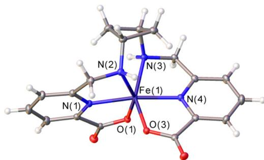
**Fig. 1** X-ray crystal structure of  $[Fe(1,3-CBuDEDPA)](PF_6) \cdot H_2O$  with ellipsoids plotted at the 50% probability level. Water molecules and anions were omitted for simplicity. Bond distances of the metal coordination sphere (Å):  $Fe(1)–N(1)$ , 2.0664(13);  $Fe(1)–N(2)$ , 2.1975(13);  $Fe(1)–N(3)$ , 2.2015(13);  $Fe(1)–N(4)$ , 2.0628(13);  $Fe(1)–O(1)$ , 1.9746(11);  $Fe(1)–O(3)$ , 1.9692(11).
