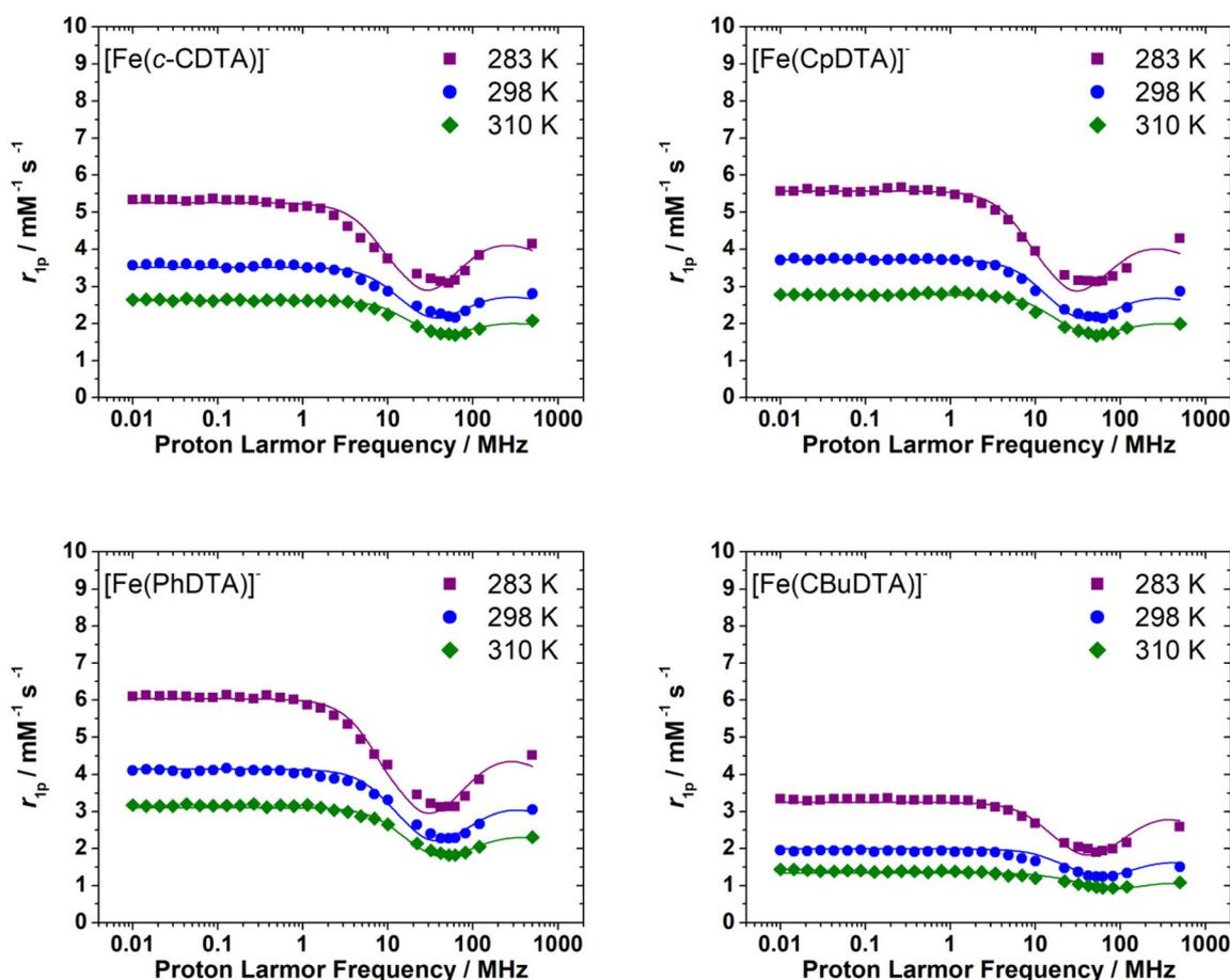
Fig. 6  $^1\text{H}$  NMRD profiles recorded for  $[\text{Fe}(c\text{-CDTA})]^-$  (3.3 mM, pH 6.0),  $[\text{Fe}(\text{CpDTA})]^-$  (5.9 mM, pH 6.1),  $[\text{Fe}(\text{PhDTA})]^-$  (4.9 mM, pH 7.2) and  $[\text{Fe}(1,3\text{-CBuDTA})]^-$  (4.8 mM, pH = 5.5) at different temperatures. The solid lines represent the fits of the data, as described in the text.
