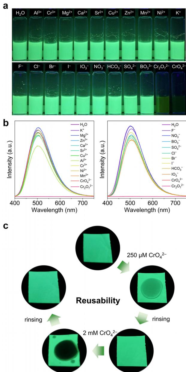
**Fig. 6** (a) Photographs of **Th-BCTPE-1** immersed in different cation and anion solutions under UV irradiation. (b) Photoluminescence spectra of **Th-BCTPE-1** immersed in different cation and anion solutions. (c) Photographs of a **Th-BCTPE-1**@PVDF membrane showing its excellent reusability.
