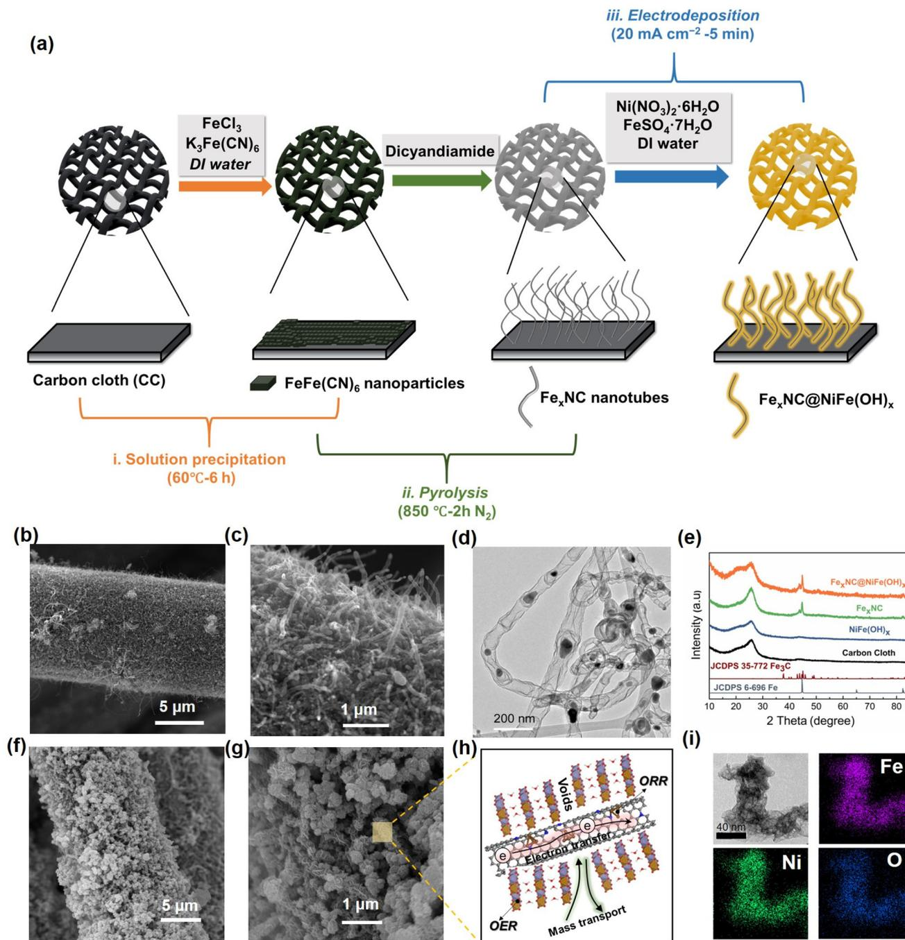
**Fig. 1** (a) Schematic illustration of the synthesis route for  $\text{Fe}_x\text{NC@NiFe(OH)}_x$ . (b–d) SEM and TEM images of  $\text{Fe}_x\text{NC}$ . (e) XRD patterns of as-prepared electrodes. (f and g) SEM images of  $\text{Fe}_x\text{NC@NiFe(OH)}_x$  and (h) the corresponding schematic diagram. (i) TEM image of  $\text{Fe}_x\text{NC@NiFe(OH)}_x$  and EDS elemental mapping images.
