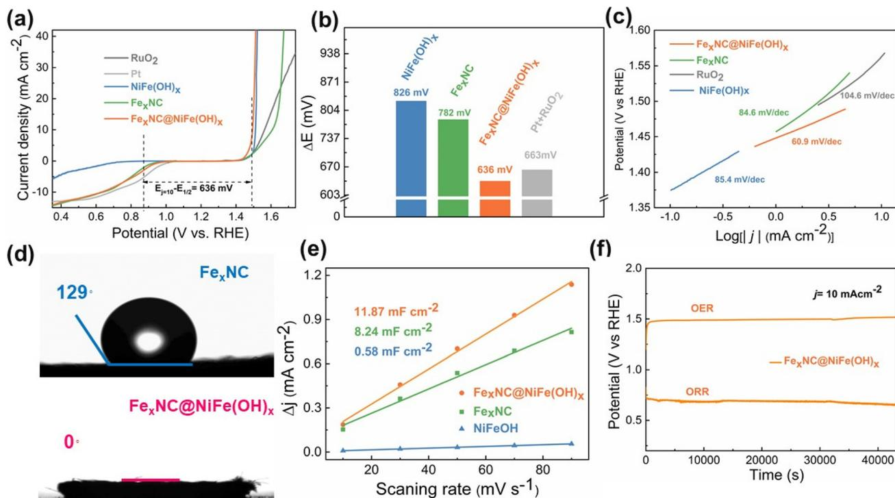
**Fig. 3** (a) The polarization curves of different electrodes. (b) Potential difference ( $\Delta E$ ) of  $\text{NiFe(OH)}_x$ ,  $\text{Fe}_x\text{NC}$ ,  $\text{Fe}_x\text{NC@NiFe(OH)}_x$ , and  $\text{Pt} + \text{RuO}_2$ . (c) OER Tafel slopes. (d) Contact angle evaluation on  $\text{Fe}_x\text{NC}$  and  $\text{Fe}_x\text{NC@NiFe(OH)}_x$ . (e) ECSA results of different electrodes. (f) The voltage-time curves of  $\text{Fe}_x\text{NC@NiFe(OH)}_x$  at  $10 \text{ mA cm}^{-2}$ .
