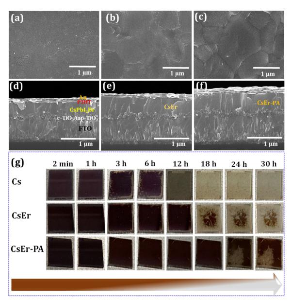
Fig. 1 SEM top view images. (a)  $CsPbl_2Br$  (Cs), (b)  $CsPb_{0.97}Er_{0.03}l_2BrCl_{0.09}$  (CsEr), (c)  $CsPb_{0.97}Er_{0.03}l_2BrCl_{0.09}$  + PABr-2 mg ml<sup>-1</sup> (CsEr-PA) perovskite thin films. SEM cross-sectional view of (d) Cs, (e) CsEr, (f) CsEr-PA-based whole IPVSC devices and (g) different time exposure dependent photographic images of the Cs, CsEr and CsEr-PA perovskite thin films (Corresponding devices stored in ambient conditions at ~25% RH without encapsulation).
