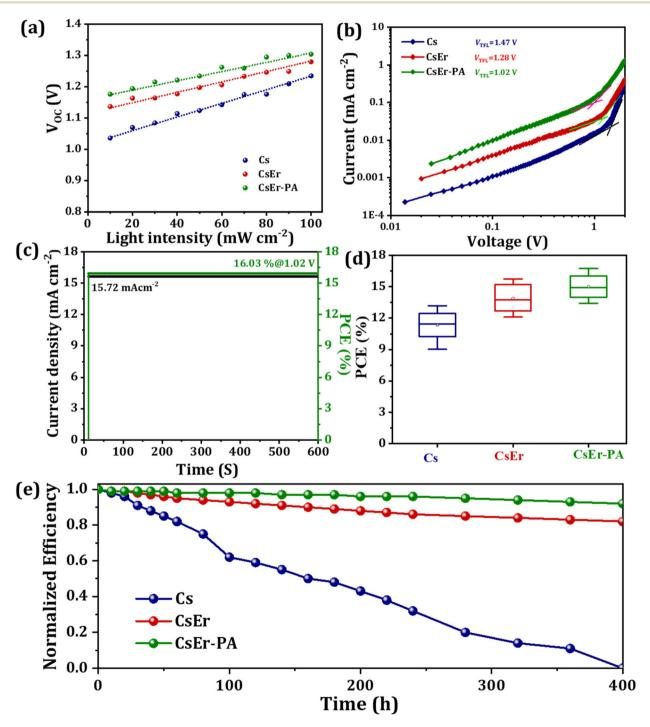
Fig. 5 (a) V<sub>OC</sub> as a function of light intensity, (b) dark current-voltage curves of electron-only devices, (c) steady-state output at the maximum power point tracking (MPPT) of the CsEr-PA-based on the IPVSC, (d) reproducibility of the Cs, CsEr and CsEr-PA-based IPVSC devices and (e) thermal long term stability of Cs, CsEr and CsEr-PA-based IPVSCs without any encapsulation under a ~25% relative humidity (RH).
