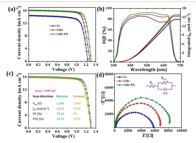
Fig. 4 (a) J-V measurements, (b) external quantum efficiency (EQE) of Cs, CsEr and CsEr-PA-based perovskite devices, (c) hysteresis of the champion CsEr-PA-based device, (d) EIS analysis of the Cs, CsEr, CsEr-PA-based perovskite devices.
