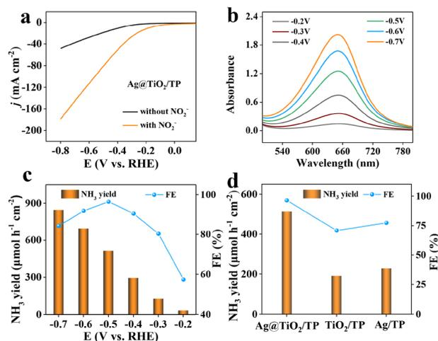
**Fig. 3** (a) LSV curves of Ag@TiO<sub>2</sub>/TP in 0.1 M NaOH with/without 0.1 M NO<sub>2</sub><sup>−</sup>. (b) UV-vis spectra of Ag@TiO<sub>2</sub>/TP at various potentials. (c) NH<sub>3</sub> yields and FEs of Ag@TiO<sub>2</sub>/TP at various potentials. (d) Comparison of NH<sub>3</sub> yields and FEs of Ag@TiO<sub>2</sub>/TP, TiO<sub>2</sub>/TP, and Ag/TP at −0.5 V.
