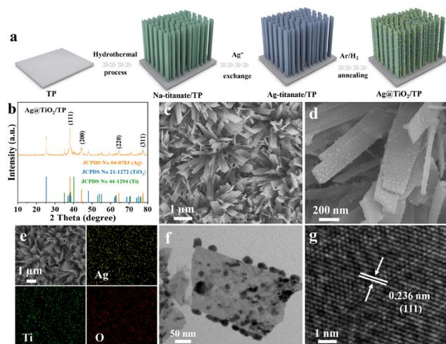
**Fig. 1** (a) Schematic illustration of the fabrication process of Ag@TiO<sub>2</sub>/TP. (b) XRD pattern and (c) and (d) SEM images of Ag@TiO<sub>2</sub>/TP. (e) SEM and corresponding elemental mapping images of Ag@TiO<sub>2</sub>/TP. (f) TEM and (g) HRTEM images of Ag@TiO<sub>2</sub>.
