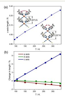
Fig. 3 Thermal expansion behaviour of compound 1 (a) Temperature dependence c-axis length. (b) Linear thermal expansion coefficients calculated from PASCal.
