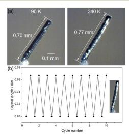
Fig. 4 Photographs of the crystal deformation of 1. (a) Expansion and shrinkage of the rod-like single crystal in the temperature range of 90-340 K. According to the result of face index, the long axis of the single crystal is parallel to the crystallographic c-axis. The crystal length increased from 0.70 to 0.77 mm upon heating. (b) Fatigue resistance test of the crystal-shape change.
