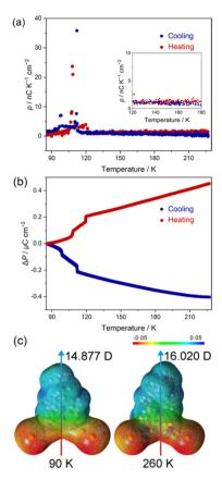
**Fig. 5** Pyroelectric effect of compound **1**. (a) Pyroelectric coefficient (p). (b) Polarization change ( $\Delta P$ ). (c) Dipole moment of the structure of part B, in which the red area represents the negative charge and the blue area represents the positive charge.
