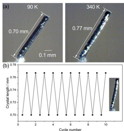
**Fig. 4** Photographs of the crystal deformation of **1**. (a) Expansion and shrinkage of the rod-like single crystal in the temperature range of 90–340 K. According to the result of face index, the long axis of the single crystal is parallel to the crystallographic *c*-axis. The crystal length increased from 0.70 to 0.77 mm upon heating. (b) Fatigue resistance test of the crystal-shape change.
