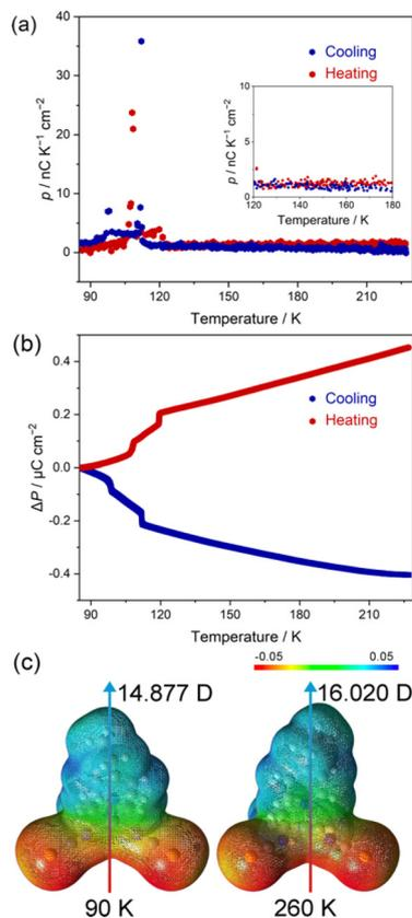
**Fig. 5** Pyroelectric effect of compound **1**. (a) Pyroelectric coefficient ( $p$ ). (b) Polarization change ( $\Delta P$ ). (c) Dipole moment of the structure of part B, in which the red area represents the negative charge and the blue area represents the positive charge.
