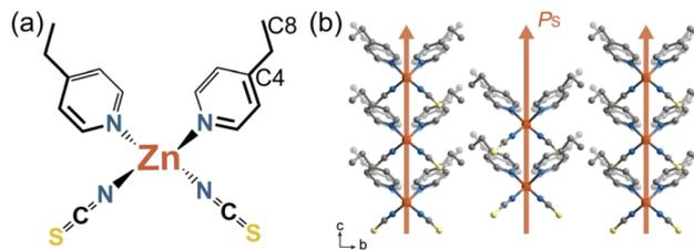
**Fig. 1** Molecular structures of compound **1**. (a) Schematic of **1**. (b) Molecular packing viewed along the  $a$ -axis at 293 K. The brown arrows indicate the direction of spontaneous polarization. Colour code: Zn (brown), N (blue), C (grey), and S (yellow). Hydrogen atoms are omitted for clarity.
