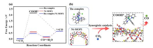
Fig. 5 The DFT results and possible mechanism. (a) Free energy profile for the CO₂RR on Ni-MOF1 and Ru complex/Ni-MOF1 (the free energy zero is set as that of a CO2 molecule in the gas phase and the catalyst). (b) Synergistic effect of a CO2 bridged photocatalytic interface of the Ru complex and Ni-MOF1.
