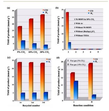
Fig. 3 CO<sub>2</sub> photoreduction performance and recycling. (a) Ni-MOF1 under different CO<sub>2</sub> concentrations. (b) Ni-MOF1 under various reaction conditions. (c) Cycling tests under 3 h of irradiation in a 10% CO2 atmosphere over Ni-MOF1. (d) The yield of CO and H<sub>2</sub> on Ni-MOF1 in real flue gas.
