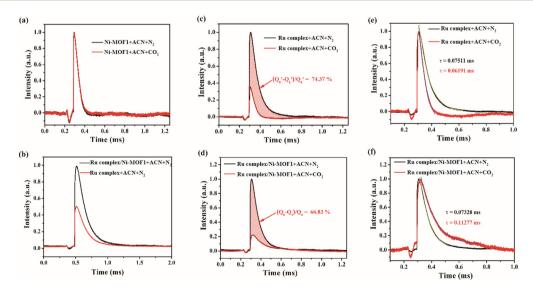
Fig. 4 The *in situ* TPV patterns of different materials in  $N_2$ -saturated ACN solution (black curve) and  $CO_2$ -saturated ACN solution (red curve). (a) Ni-MOF1. (b) Ru complex/Ni-MOF1 (black curve) and Ru complex (red curve) in  $N_2$ -saturated ACN solution. (c) Ru complex. (d) Ru complex/Ni-MOF1. Charge annihilation process of (e) the Ru complex and (f) Ru complex/Ni-MOF1.
