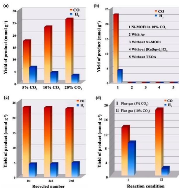
**Fig. 3** CO<sub>2</sub> photoreduction performance and recycling. (a) Ni-MOF1 under different CO<sub>2</sub> concentrations. (b) Ni-MOF1 under various reaction conditions. (c) Cycling tests under 3 h of irradiation in a 10% CO<sub>2</sub> atmosphere over Ni-MOF1. (d) The yield of CO and H<sub>2</sub> on Ni-MOF1 in real flue gas.
