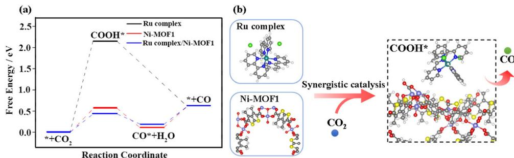
**Fig. 5** The DFT results and possible mechanism. (a) Free energy profile for the CO<sub>2</sub>RR on Ni-MOF1 and Ru complex/Ni-MOF1 (the free energy zero is set as that of a CO<sub>2</sub> molecule in the gas phase and the catalyst). (b) Synergistic effect of a CO<sub>2</sub> bridged photocatalytic interface of the Ru complex and Ni-MOF1.
