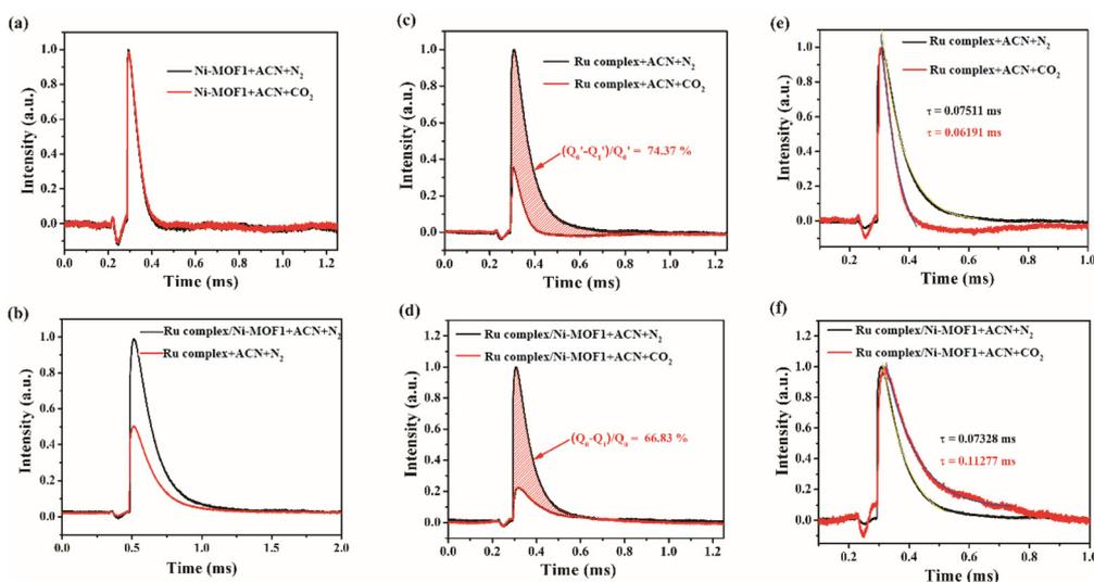
**Fig. 4** The *in situ* TPV patterns of different materials in N<sub>2</sub>-saturated ACN solution (black curve) and CO<sub>2</sub>-saturated ACN solution (red curve). (a) Ni-MOF1. (b) Ru complex/Ni-MOF1 (black curve) and Ru complex (red curve) in N<sub>2</sub>-saturated ACN solution. (c) Ru complex. (d) Ru complex/Ni-MOF1. Charge annihilation process of (e) the Ru complex and (f) Ru complex/Ni-MOF1.
