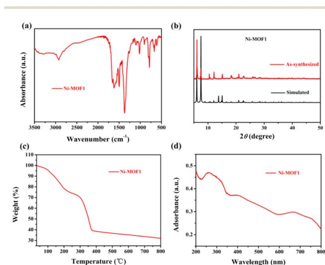
**Fig. 2** Basic characterization of Ni-MOF1. (a) Infrared (IR) spectra. (b) Powder X-ray diffraction (PXRD) (black curve: single-crystal simulation and red curve: experimental synthesis). (c) TGA curves. (d) UV-vis diffuse reflectance spectra.
