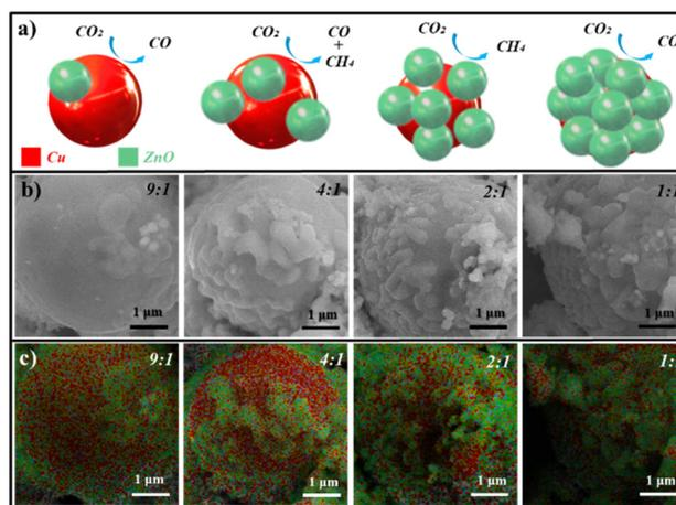
**Fig. 1** (a) Schematic diagrams of the designed heterointerface structures. Red and green balls represent metal Cu and ZnO, respectively. (b) SEM images and (c) overlap mapping pictures of the Cu–ZnO catalysts with different heterointerfaces. The Cu : Zn ratios were 9 : 1, 4 : 1, 2 : 1, and 1 : 1, respectively. Red and green areas represent the element distribution of Cu and Zn, respectively. The ratios were acquired from ICP tests.
