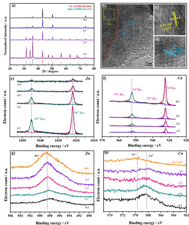
**Fig. 2** (a) XRD patterns of different Cu : Zn ratios of Cu–ZnO catalysts. (b) HRTEM of 2Cu–1ZnO, together with patterns derived from the (c) yellow and (d) blue areas. XPS spectra of the selected samples: (e) Zn 2p, (f) Cu 2p, (g) Zn Auger peaks, and (h) Cu Auger peaks, respectively.
