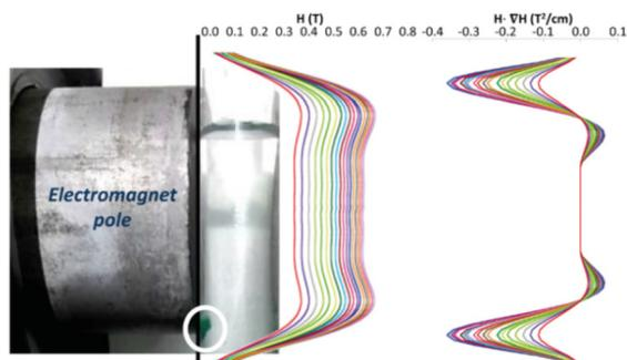
Fig. 7 Magnetic field profile [ $H$  and  $H \cdot \nabla(H)$ ] on the electromagnet pole along the dashed line. The different colours refer to the applied intensity current: increasing from 0.0 to 2.5 A (step: 0.1 A).
