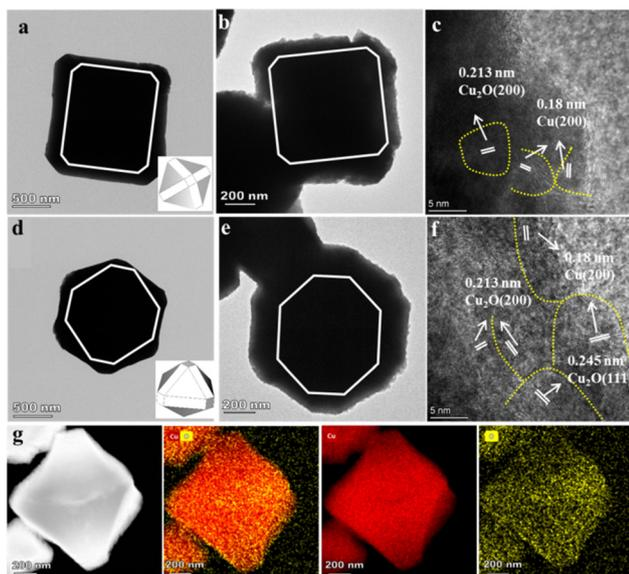
**Fig. 1** Structural characterization of catalysts. The TEM images of T-Cu<sub>2</sub>O viewed along the (a) [100] and (d) [111] directions, and the (b) and (e) TEM images, (c) and (f) HR-TEM images, (g) HAADF-STEM and elemental mapping images (Cu species were in red, and O species were in yellow) of surface-reconstructed T-Cu<sub>2</sub>O samples after reduction at  $-1.1$  V vs. RHE.
