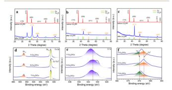
Fig. 2 XRD patterns of catalysts: (a) F-Cu<sub>2</sub>O, (b) O-Cu<sub>2</sub>O and (c) T-Cu<sub>2</sub>O. XPS spectra of (d) Cu 2p, (e) O 1s and (f) Cu LMM of F-Cu<sub>2</sub>O, O-Cu<sub>2</sub>O and T-Cu<sub>2</sub>O after CO<sub>2</sub>RRs at -1.1 V vs. RHE until stable.
