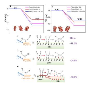
Fig. 5 Adsorption energies of (a) CO and (b) C<sub>2</sub>H<sub>4</sub> on F-Cu<sub>2</sub>O/Cu(100), O-Cu<sub>2</sub>O/Cu(111) and T-Cu<sub>2</sub>O/Cu(111)/(100) catalysts. Formation of C<sub>2</sub>H<sub>4</sub> on (c) O-Cu<sub>2</sub>O/Cu(111), (d) F-Cu<sub>2</sub>O/Cu(100) and (e) T-Cu<sub>2</sub>O/Cu(111)/ (100) catalysts.
