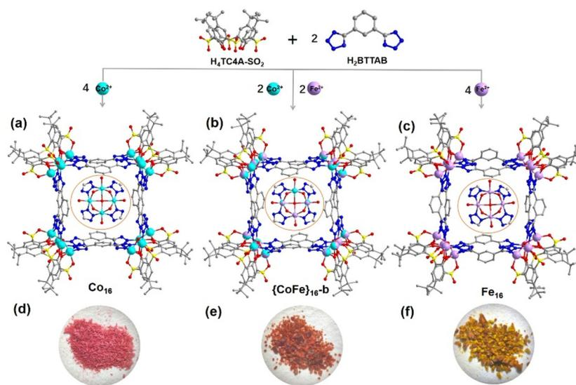
**Fig. 1** Schematic illustration of the syntheses of Co<sub>16</sub>, {CoFe}<sub>16</sub>-b and Fe<sub>16</sub>: (a–c) the crystal structures and the coordination mode of metal ions (inset) and (d–f) the photograph of the crystals. Hydrogen atoms are omitted for clarity.
