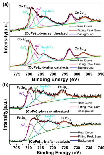
**Fig. 3** High-resolution Co 2p (a) and Fe 2p (b) XPS spectra of the as-synthesized {CoFe}<sub>16</sub>-b and {CoFe}<sub>16</sub>-b after catalysis (after LSV).
