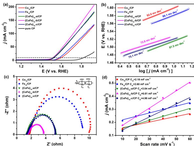
**Fig. 2** (a) OER polarization curves and (b) Tafel plots for the different electrocatalysts in 1 M KOH solution. (c) Nyquist plots for different electrocatalysts recorded at 1.53 V vs. RHE (inset: the equivalent circuit model for electrochemical impedance tests). (d) Plots of the charging current density against scan rates of different catalysts for determining the ECSA.
