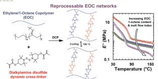
Novel covalent adaptable networks (CANs) of ethylene/1-octene copolymers (EOCs) made by free-radical processing: comparison of structure– property relationships of EOC CANs with EOC thermosets
