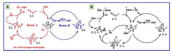
Fig. 5 Possible thiourethane exchange mechanisms (schematic). A: Exchange mechanisms occurring via nucleophilic (route A) and basic (route B) catalysis. B: Thiourethane exchange mechanism for a combined nucleophilic and basic catalyst, DBN. Reproduced from ref. 80 with permission from Elsevier, copyright 2020.
