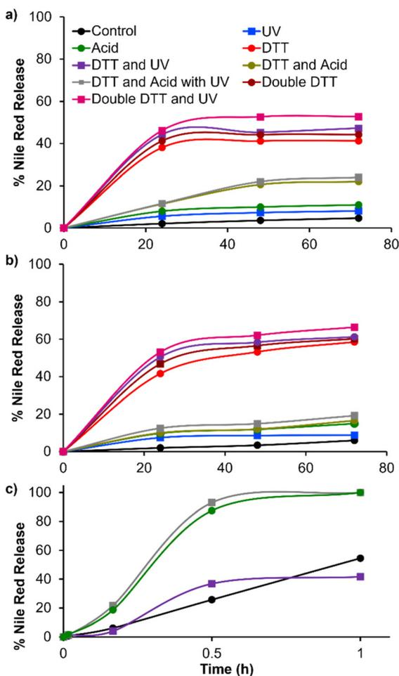
**Fig. 4** Nile red release profiles for spherical TORC-NGs (a), worm-like TORC-NGs (b) and non-CCL nanosphere (c) upon application of various stimuli simultaneously (legend applies to all plots; control = no stimuli; acid = adjusted to pH 4 with HCl/H<sub>2</sub>O; DTT = addition of 66.2 mM DTT for spherical TORC-NG and 51.1 mM DTT for worm-like TORC-NG; UV = 1 h irradiation with 254 nm UV light).
