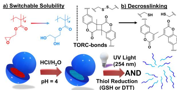
**Fig. 1** Multi-responsive TORC-NG materials, synthesized in one-pot via PhotoATR-PISA, which can fully disassemble only when first exposed to acidic aqueous environments (pH = 4; a) followed by UV-C irradiation ( $\lambda = 254$  nm) and thiol reducing agents (b).
