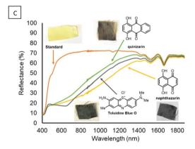
Fig. 5 (A–C) Reflectance spectra and photographs of dyed Kevlar samples, and the corresponding dye structures for each sample.
