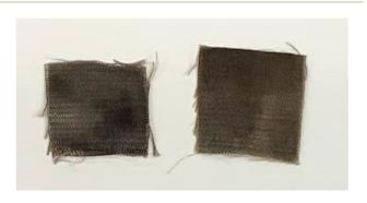
Fig. 7 Stained Kevlar sample before (left) and after (right) simulated laundering.
