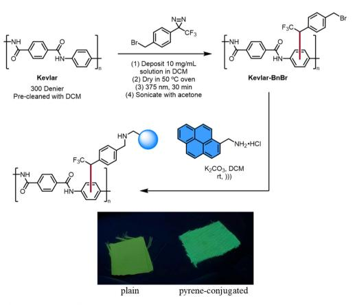
Fig. 4 Attachment of a fluorescent dye to Kevlar.
