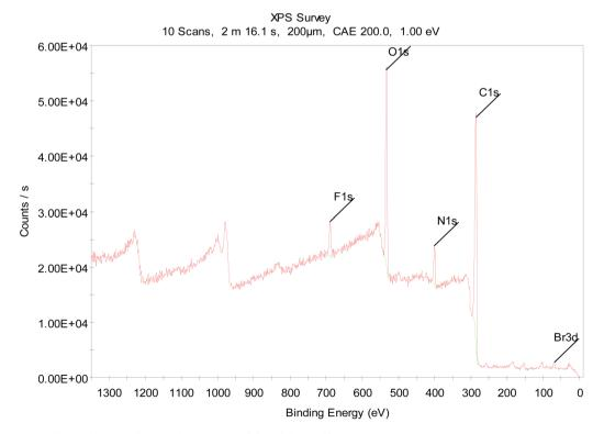
Fig. 2 XPS spectrum of Kevlar functionalized with compound 2 (see Scheme 2).
