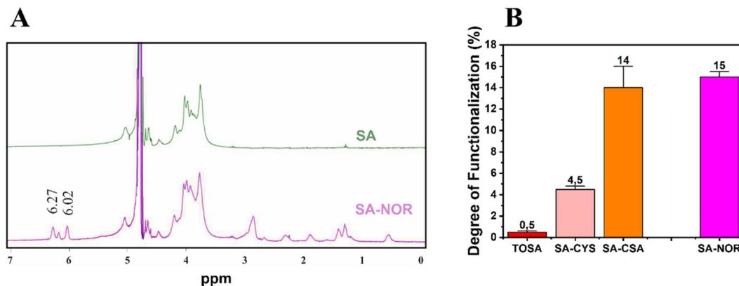
Fig. 3  $^1\text{H-NMR}$  spectra of SA-NOR and sodium alginate SA (A). Calculated degree of functionalization, obtained by the Ellman's reagent method for the thiolated monomers and by integration of the NMR peaks for SA-NOR (B).
