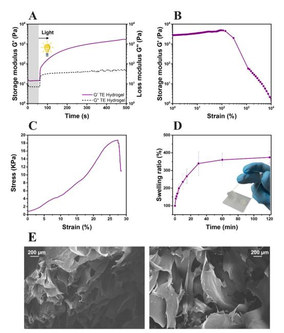
Fig. 4 Photorheology (A), amplitude sweep (B), compression test (C) and swelling kinetics (D) of the thiol-ene hydrogel (TE hydrogel). Field Emission Scanning Electron Microscopy (FESEM) of the TE hydrogels; scale bar 200 µm (E).
