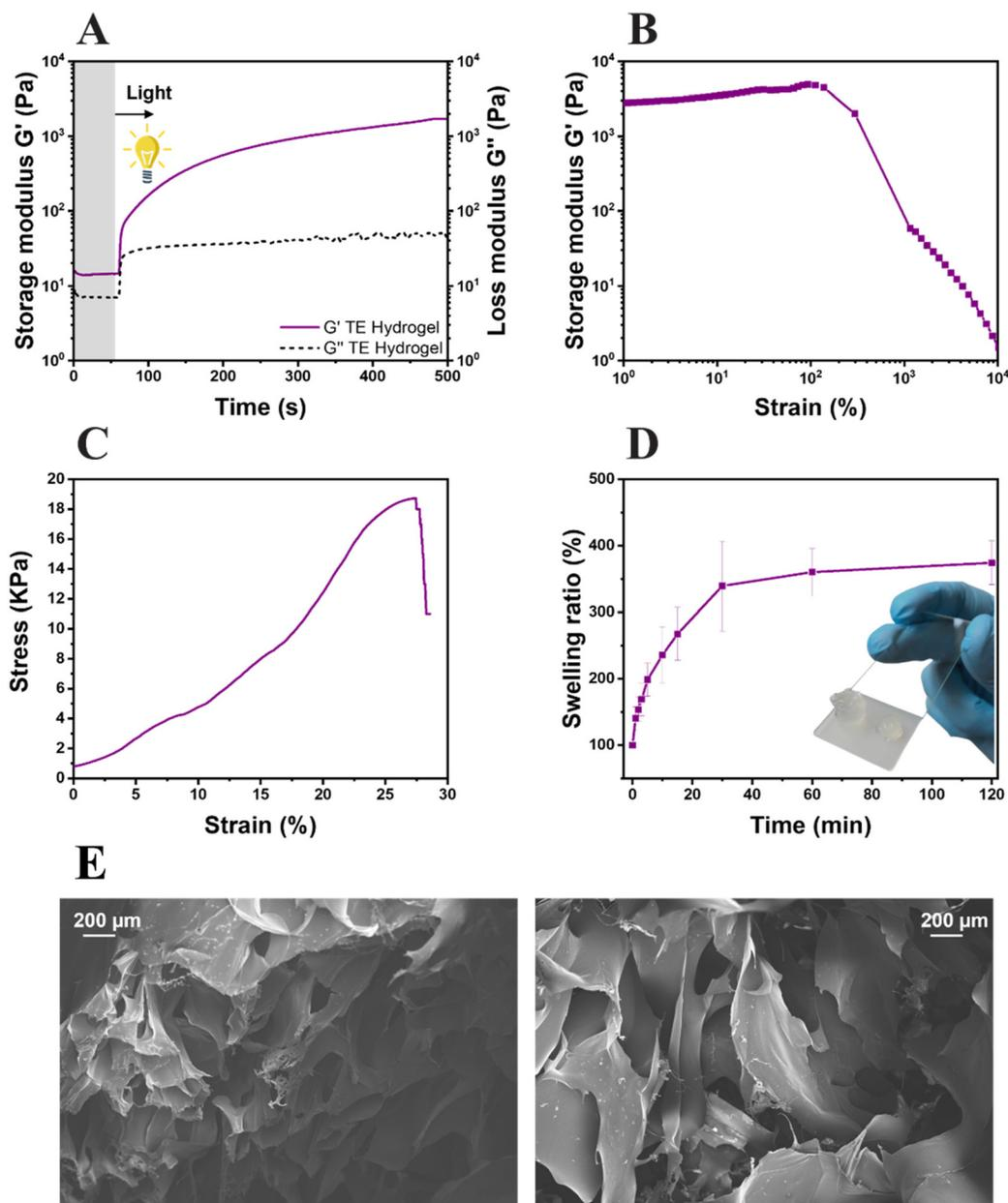
**Fig. 4** Photorheology (A), amplitude sweep (B), compression test (C) and swelling kinetics (D) of the thiol–ene hydrogel (TE hydrogel). Field Emission Scanning Electron Microscopy (FESEM) of the TE hydrogels; scale bar 200  $\mu\text{m}$  (E).
