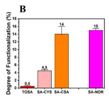
Fig. 3 <sup>1</sup>H-NMR spectra of SA-NOR and sodium alginate SA (A). Calculated degree of functionalization, obtained by the Ellman's reagent method for the thiolated monomers and by integration of the NMR peaks for SA-NOR (B).
