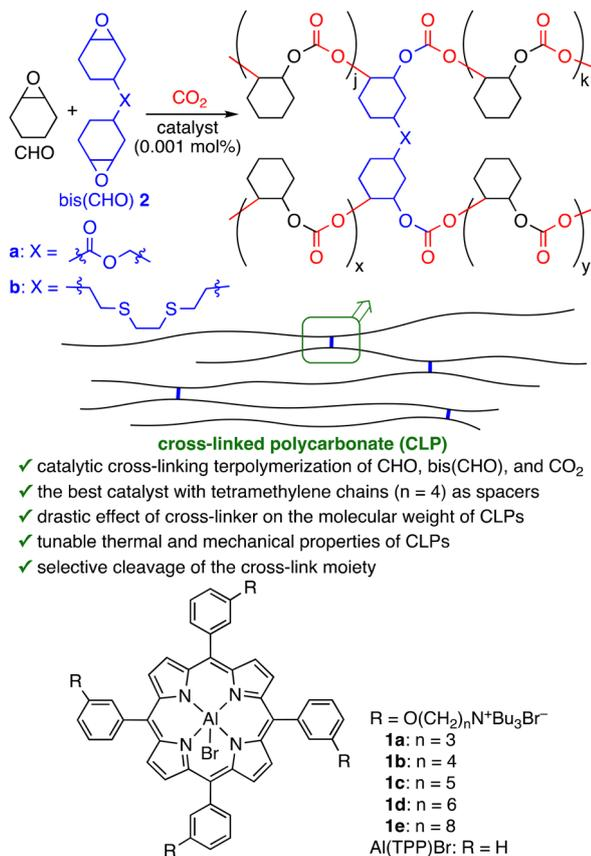
**Fig. 1** Terpolymerization of CHO, bis(CHO) **2**, and CO<sub>2</sub> catalyzed by the aluminum porphyrin catalysts.
