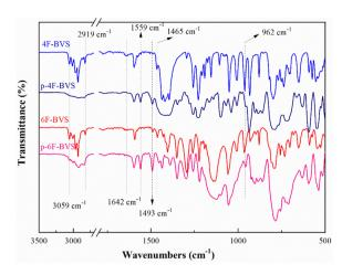
Fig. 4 FI-IR spectra of 4F-BVS and 6F-BVS before and after curing.
