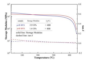
Fig. 6 DMA curves of p-4F-BVS and p-6F-BVS.
