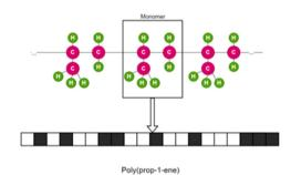
**Fig. 2** Fingerprint of poly(prop-1-end) monomer. The black and white boxes denote the presence or count of some pre-defined structures or those that correspond to some polymer properties.
