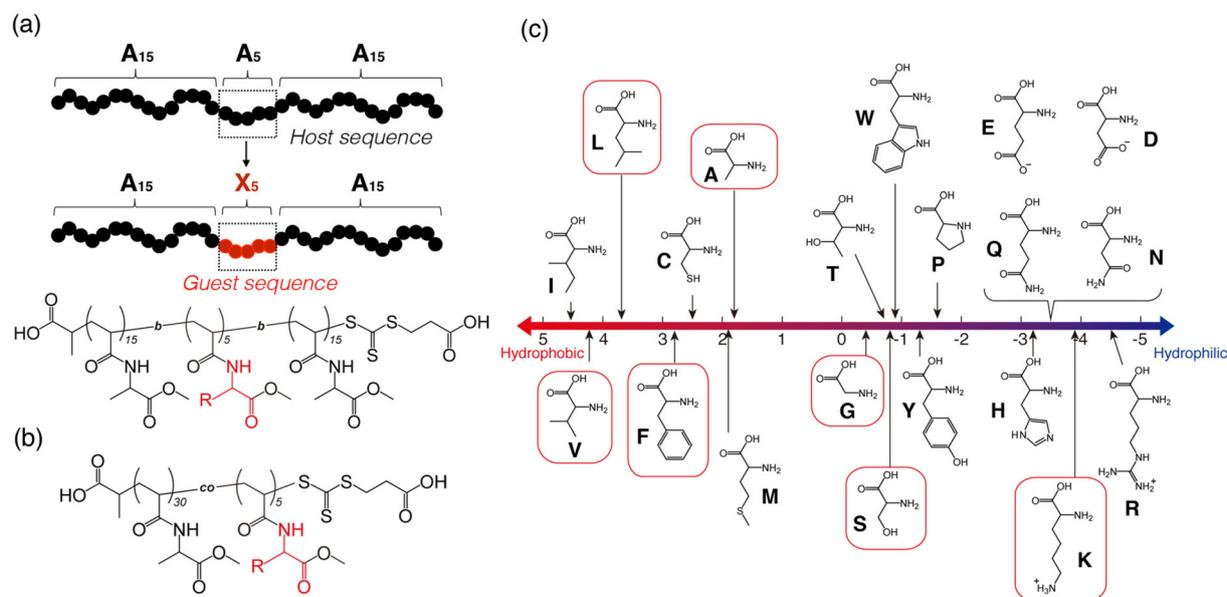
**Fig. 1** Chemical structures of thermo-responsive amino acid-derived vinyl polymers (a) A<sub>15</sub>-b-X<sub>5</sub>-b-A<sub>15</sub> and (b) A<sub>30</sub>-co-X<sub>5</sub>, based on host-guest strategy. (c) Hydropathy indices of constituent amino acids for vinyl monomer library. The amino acids indicated within the red square are the seven components used in this study.
