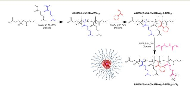
$\begin{tabular}{ll} Scheme 1 & Synthesis of p(DMAEA-stat-DMAEMA)_{25}-b-NAM_{15}-b-CL_3 star copolymer by the arm-first approach. \end{tabular}$
