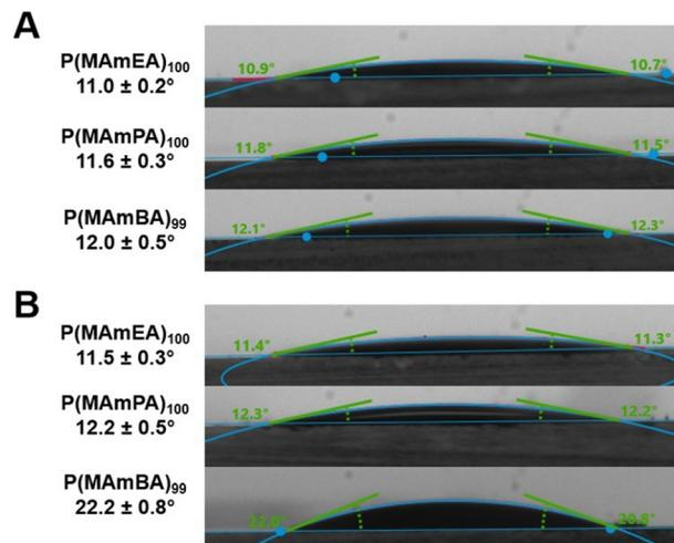
Fig. 5 (A) Water contact angle images of P(MAmEA)<sub>100</sub>, P(MAmPA)<sub>97</sub> and P(MAmBA)<sub>99</sub> at 25 °C; (B) water contact angle images of P(MAmEA)<sub>100</sub>, P(MAmPA)<sub>97</sub> and P(MAmBA)<sub>99</sub> at 75 °C.
