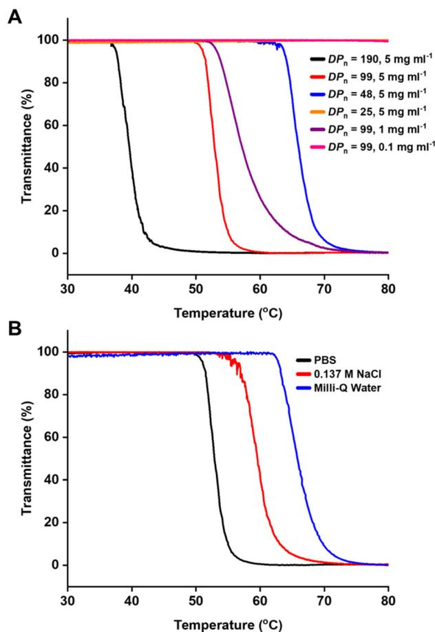
**Fig. 4** Turbidity measurements of (A) PBS solutions of P(MAmBA) of different DP<sub>n</sub> and concentrations; and (B) P(MAmBA)<sub>99</sub> solutions in different media (5 mg ml<sup>-1</sup>).
