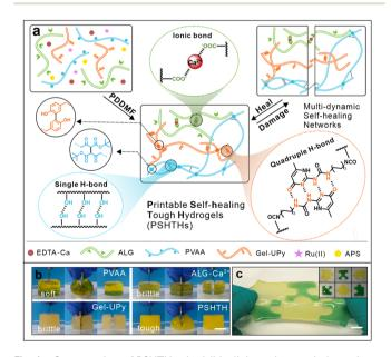
Fig. 1 Construction of PSHTHs *via* visible-light orthogonal photochemistry design. (a) The proposed schematic illustration for preparing multinetwork self-healing hydrogels. Digital images of (b) PSHTH and hydrogels with a single component and (c) self-healing property of 3D printed PSHTH patterns (scale bar: 1 cm).
