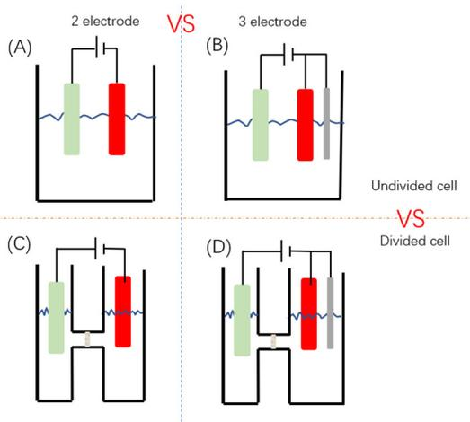
**Fig. 1** Schematic depiction of common electrochemical cell configurations including divided (C and D) and undivided configurations (A and B) for; potentiostatic reactions (B and D) consisting of a working (red), counter (green) and reference (grey) electrode; galvanostatic reactions (A and C) consisting of a working (red), counter (green) electrodes.
