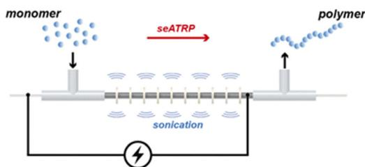
**Fig. 10** Schematic representation of continuous-flow self-supported seATRP using a sonicated microreactor. Reproduced from ref. 135 with permission from the Royal Society of Chemistry, copyright 2022.
