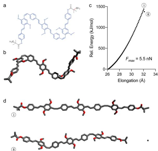
**Fig. 2** Structure of **7'** used for CoGEF simulations with constrained atoms marked in bold and scissile bond highlighted in red (a), along with its energy minimized structure (b). The evolution of energy upon simulated elongation (CoGEF, DFT B3LYP/6-31G\*) of this model (c) reveals the most elongated (E<sub>max</sub>) and post-scission structures (d).
