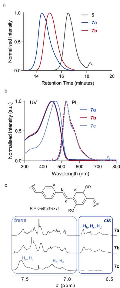
**Fig. 1** SEC traces (a), UV-PL spectra (b), and partial <sup>1</sup>H NMR spectra (500 MHz, CD<sub>2</sub>Cl<sub>2</sub>) (c) of pre- and post-sonication polymers **7a** and **7b** respectively, along with all-*trans* reference polymer **7c**. Spectra aligned on the -OCH<sub>3</sub> peak of PMMA.
