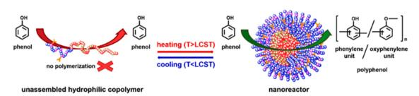
Fig. 3 Enzymatic polymerization of phenolic compounds catalyzed by HRP within nanoreactors of thermo-responsive diblock copolymer. Reprinted with permission from ref. 38. Copyright 2022 The Royal Society of Chemistry.
