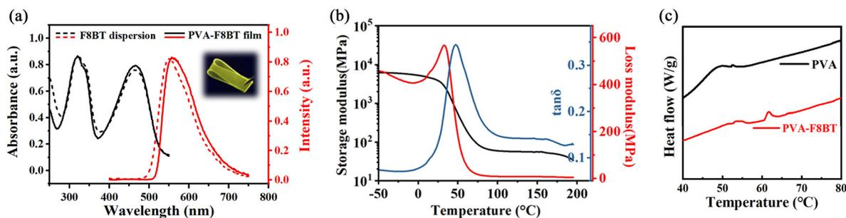
**Fig. 5** (a) UV-vis and luminescence spectra of the F8BT dispersion and the PVA-F8BT film (inset is the photo of the typical PVA-F8BT film under 365 nm UV light excitation); (b) DMA curves of the typical PVA-F8BT film; and (c) DSC curves of PVA and PVA-F8BT.
