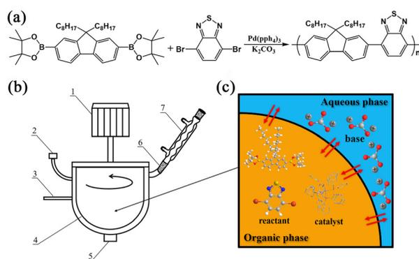
**Fig. 1** (a) Reaction scheme of the synthesis of F8BT *via* the Suzuki cross-coupling reaction. (b) Inner circulation RPB reactor with the following components: 1, rotor; 2, injection inlet; 3,  $\text{N}_2$  inlet; 4, thermostatic bath; 5, discharge hole; 6, feed inlet; and 7, condenser. (c) Schematic diagram of the reaction at the interface between organic phase and aqueous phase of the tiny reaction unit of droplet.
