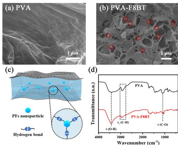
**Fig. 4** SEM images of (a) PVA and (b) PVA-F8BT (the red circles indicate the nanoparticles of F8BT in the composite); (c) schematic diagram of hydrogen bond cross-linking of F8BT nanoparticles in the PVA network structure; and (d) FTIR spectra of PVA and the PVA-F8BT nanocomposite.
